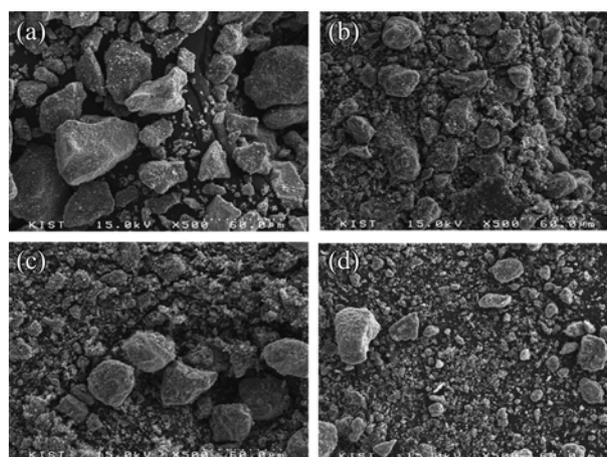
**Figure 4.** SEM images of the recycled LiFePO<sub>4</sub> and the original LiFePO<sub>4</sub> cathode materials (a): original LiFePO<sub>4</sub>, (b): recycled LiFePO<sub>4</sub> at 400 °C, (c): 500 °C, (d): 600 °C.
