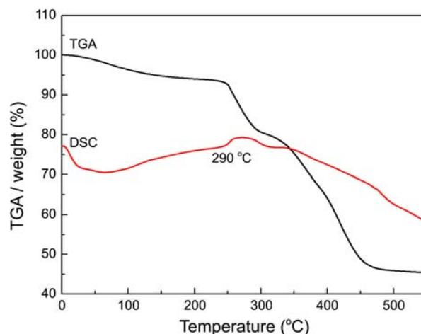
**Figure 2.** TGA and DSC curves of CMC and SBR binders.
