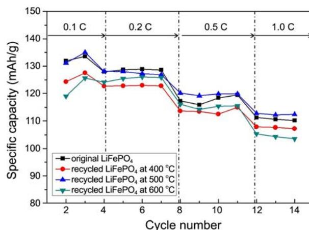
**Figure 9.** The cycling performances of the recycled LiFePO<sub>4</sub> and the original LiFePO<sub>4</sub> cathode.
