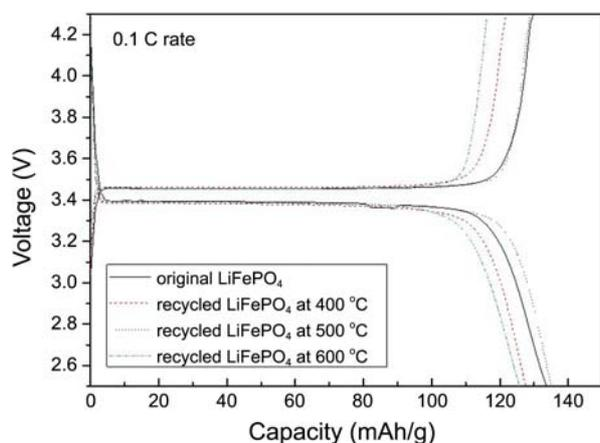
**Figure 5.** The charge/discharge voltage curves of the recycled LiFePO<sub>4</sub> and the original LiFePO<sub>4</sub> cathode at 0.1C rate.
