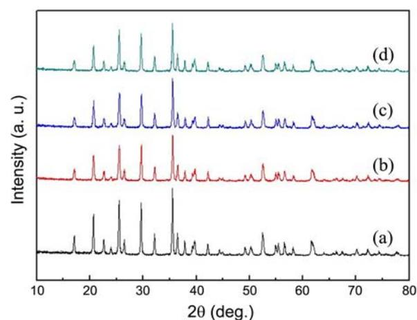
**Figure 3.** XRD pattern of the recycled LiFePO<sub>4</sub> and the original LiFePO<sub>4</sub> cathode materials (a): original LiFePO<sub>4</sub>, (b): recycled LiFePO<sub>4</sub> at 400 °C, (c): 500 °C, (d): 600 °C.
