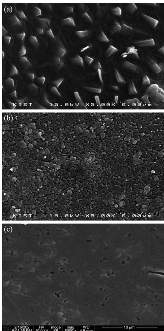
**Figure 8.** SEM images of CMC and SBR binders pyrolyzed at different temperatures (a): 400 °C, (b): 500 °C, (c): 600 °C).
