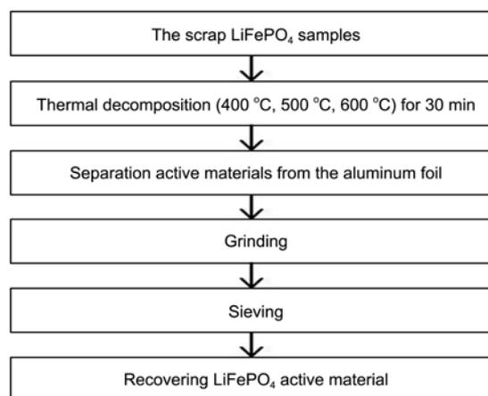
**Figure 1.** Flow diagram of the recycling process of LiFePO<sub>4</sub> cathode materials.
