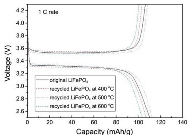
**Figure 6.** The charge/discharge voltage curves of the recycled LiFePO<sub>4</sub> and the original LiFePO<sub>4</sub> cathode at 1C rate.
