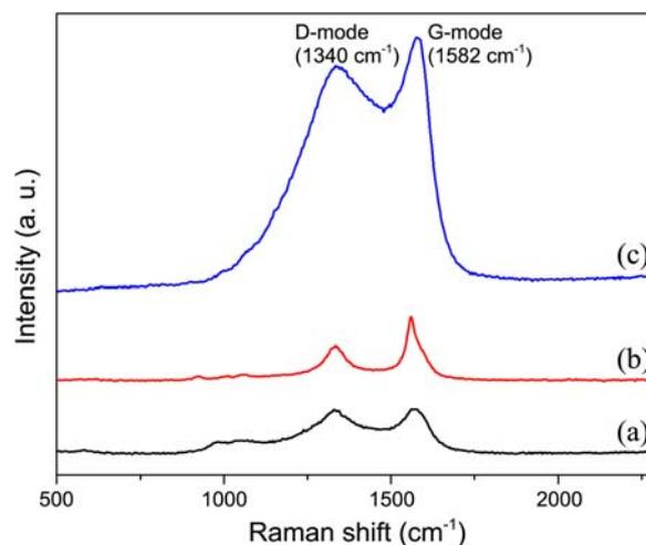
**Figure 7.** Raman spectrum of CMC and SBR binder decomposed at different temperatures (a): 400 °C, (b): 500 °C, (c): 600 °C.
