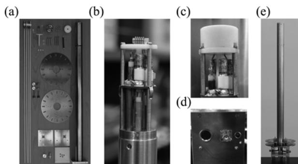
**Figure 1.** The 800 MHz NB lab-built strip-shield low- $\epsilon$  solid-state NMR probe. (a) Parts of the probe assembly. (b) The completed probe head, the strip shield was used to prevent heating of the bicelle sample and the coil. (c) PTFE coil cap for the sample. (d) Probe heat sensor and heater for temperature control. (e) The whole probe.
