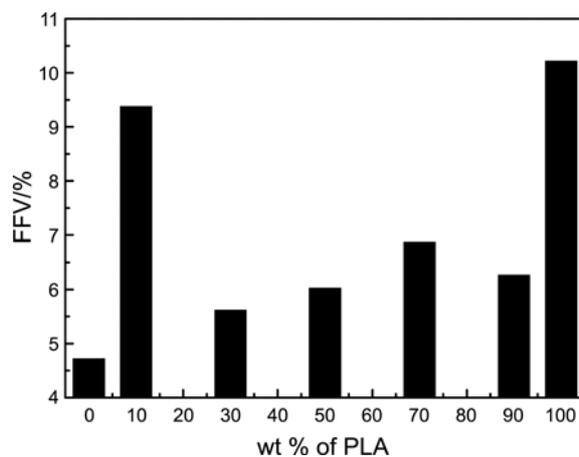
**Figure 4.** The simulated FFV of the PET/PLA blends measured by a probe of size of  $\text{CO}_2$ .
