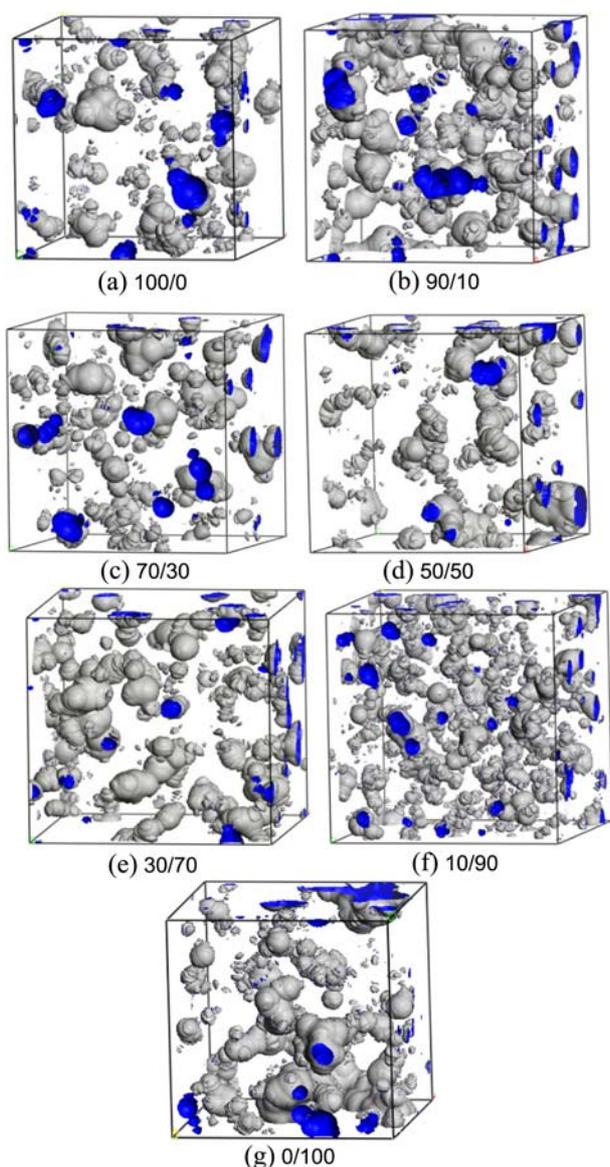
**Figure 3.** Simulated morphologies of free volumes in the well-equilibrated models of PET/PLA blends.
