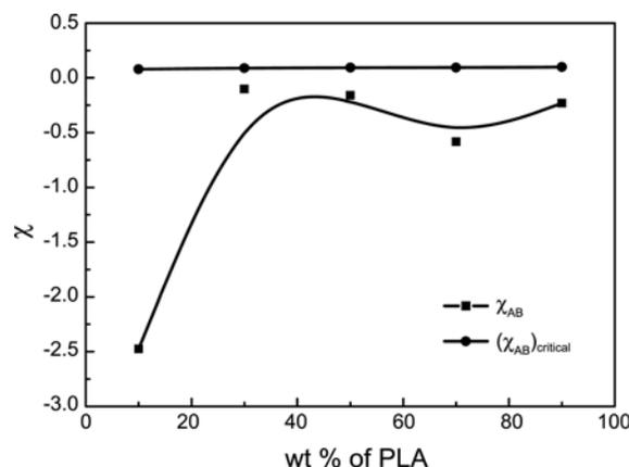
**Figure 2.** Flory-Huggins interaction parameter vs weight fraction of PLA.
