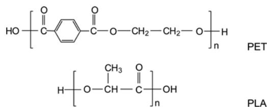
**Figure 1.** Chemical structures of PET and PLA.
