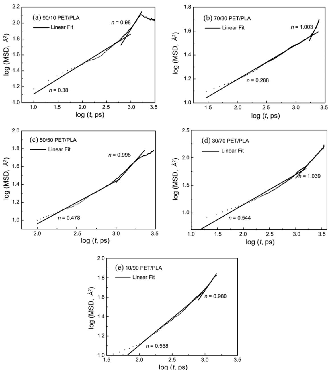
**Figure 5.** Log(MSD) vs log(*t*) plots for the diffusion of CO<sub>2</sub> in PET/PLA blends.
