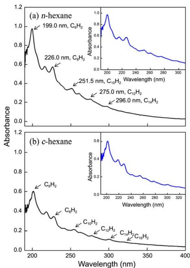
**Figure 2.** Typical UV absorption spectrum of a polyne solution produced by laser ablation of a graphite target in *n*-hexane (a) and *c*-hexane (b) at 1064 nm (20 mJ/pulse).
