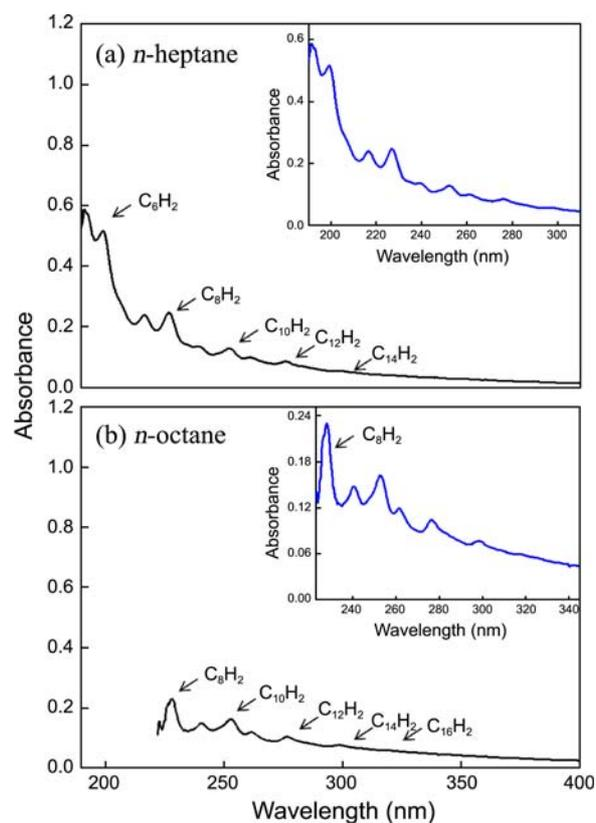
**Figure 3.** Typical UV absorption spectrum of a polyne solution produced by laser ablation of a graphite target in *n*-heptane (a) and *n*-octane (b) at 1064 nm (20 mJ/pulse).
