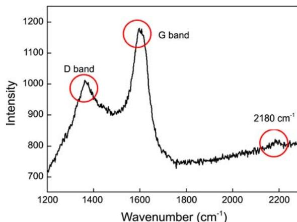
**Figure 1.** Raman spectrum of polyynes solution prepared by laser ablation of graphite target in *n*-hexane at 1064 nm.
