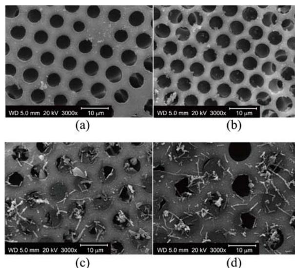
**Figure 6.** Typical SEM images showing the effect of loaded electrical field on the formation of the PANI-MWCNT/PS composite film obtained by the loaded voltage of 1.0 V. (a), (b), (c), and (d) show the SEM images of PANI-MWCNT/PS composite with the polymerization time of 1, 2, 6, and 8 h, respectively. 3 wt % of MWCNT was used.
