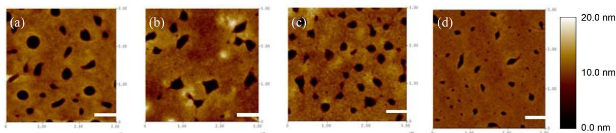
**Figure 4.** AFM height images of PFTT/PC<sub>71</sub>BM layers in photovoltaic devices with various weight ratios of PFTT to PC<sub>71</sub>BM: (a) 1:1, (b) 1:2, (c) 1:3, and (d) 1:4 (the scale bar is 500 nm).
