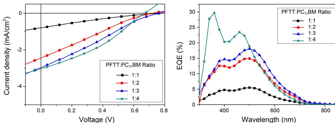
**Figure 3.** (Left) J-V curves and (right) EQE spectra of PFTT-based solar cells under illumination from an AM 1.5G solar simulator ( $100 \text{ mW/cm}^2$ ).
