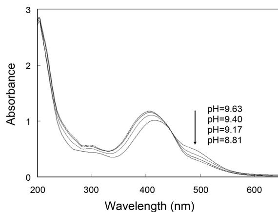
**Figure 3.** UV-vis absorption spectra of 109  $\mu\text{M}$  catechin in basic buffer solutions 19 hours after the addition of catechin to the buffer solution.
