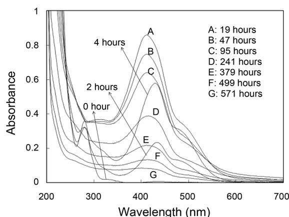
**Figure 2.** UV-vis absorption spectra of 91  $\mu\text{M}$  catechin in a buffer solution at pH = 8.81 at various times.
