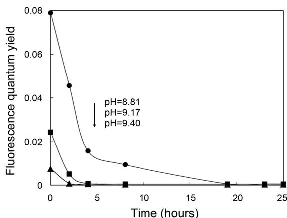
**Figure 5.** Fluorescence quantum yields of the 91  $\mu\text{M}$  catechin as a function of the storage time at various pH values for the basic buffer solution.
