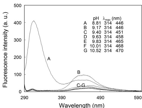
**Figure 4.** Fluorescence spectra (excitation at 280 nm) of 91  $\mu\text{M}$  catechin in basic buffer solutions 4 hours after adding the catechin to the solution.
