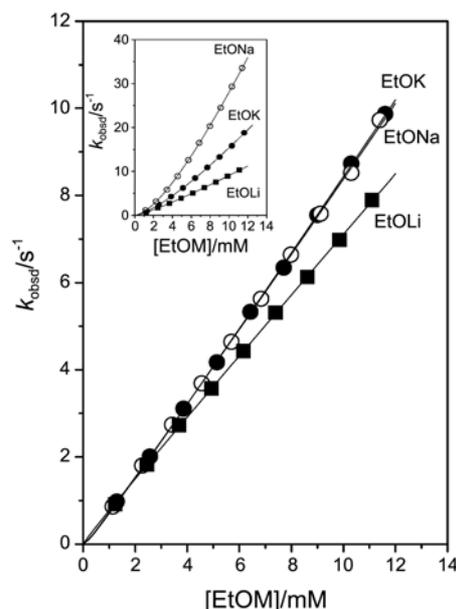
**Figure 1.** Plots of  $k_{obsd}$  vs. [EtOM] for reactions of 4-nitrophenyl nicotinate **5** and picolinate **4** (inset) with EtOK (●), EtONa (○), and EtOLi (■) in anhydrous EtOH at  $25.0 \pm 0.1$  °C. Data for the reactions of **4** were taken from ref. 10b.
