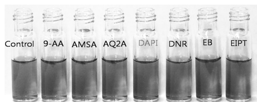
Figure 3. Color changes in gold nanoparticle substrates 45 minutes after the addition of DNA binding molecules.
