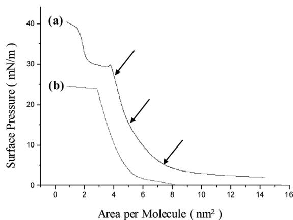
**Figure 5.** Surface pressure-area isotherms of dumbbell-shaped molecules. (a)  $\pi$ -A isotherms of molecule **1** and (b)  $\pi$ -A isotherms of molecule **2** with deposition points indicated by arrows.
