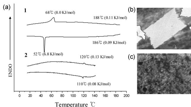
**Figure 1.** (a) DSC curves of dumbbell-shaped molecules **1** and **2**. (b) Representative optical polarized micrograph (100 ×) of the texture exhibited by a primitive orthorhombic structure for **1**. (c) Representative optical polarized micrograph (100 ×) of the texture exhibited by nematic structure for **2** at the transition from the isotropic liquid state.
