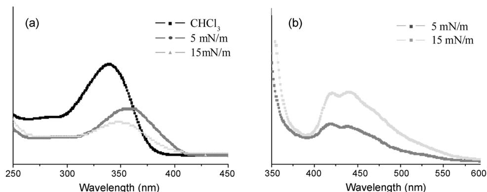
**Figure 7.** (a) Uv-vis absorption spectra of molecule **1** in chloroform, at surface pressure of 5 mN/m and at surface pressure 15 mN/m. (b) Fluorescence emission of molecule **1** at surface pressure of 5 mN/m and at surface pressure 15 mN/m.
