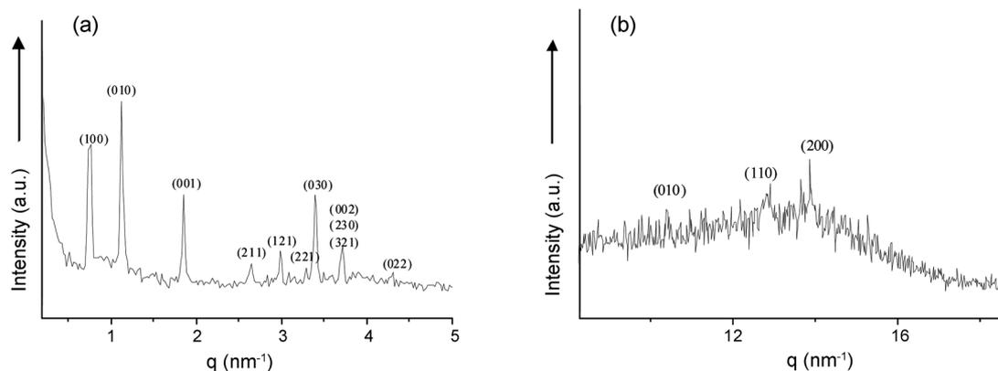
**Figure 2.** (a) Small-angle X-ray diffraction pattern of **1** measured at 55 °C, (b) wide-angle X-ray diffraction pattern of **1** measured at 55 °C.
