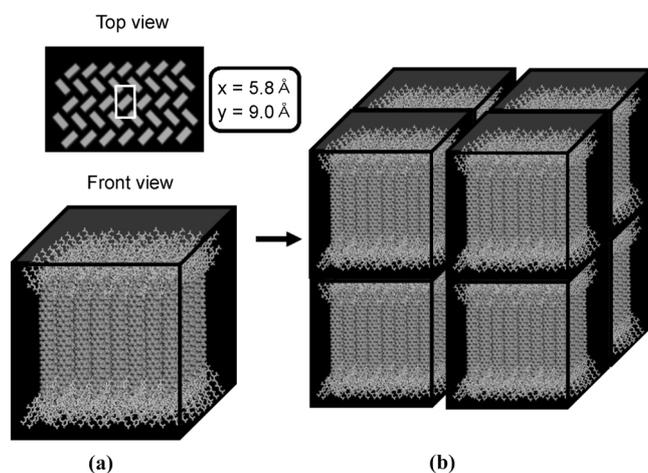
**Figure 4.** Schematic representation of (a) the self-assembly of **1** into a discrete bundle with the herringbone packing and (b) the subsequent crystallization into a primitive orthorhombic superlattice.
