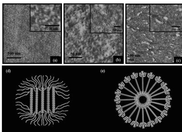
**Figure 6.** AFM topographical images of LB monolayer from molecule **1** (a) at surface pressure of 5 mN/m, (b) at surface pressure of 15 mN/m, (c) at surface pressure of 25 mN/m and schematic representation of **1** (d) self-organize into circular plate structure and (e) ring structure.
