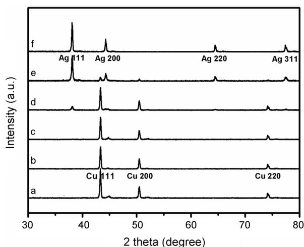
**Figure 2.** The XRD patterns of (a) pure  $\mu\text{Cu}$ , (b)  $\mu\text{Cu}@Ag(0.05)$ , (c)  $\mu\text{Cu}@Ag(0.5)$ , (d)  $\mu\text{Cu}@Ag(5)$ , (e)  $\mu\text{Cu}@Ag(50)$ , and (f) pure  $\mu\text{Ag}$  powders.
