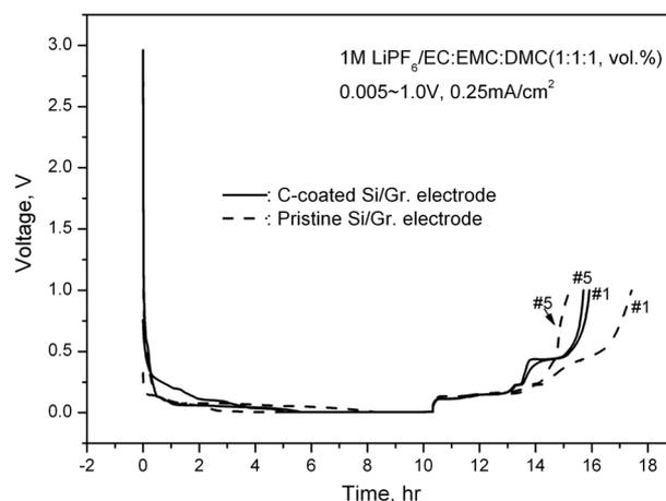
**Figure 5.** Charge/Discharge curves of C-coated Si/Gr. anode and pristine Si/Gr. anode.
