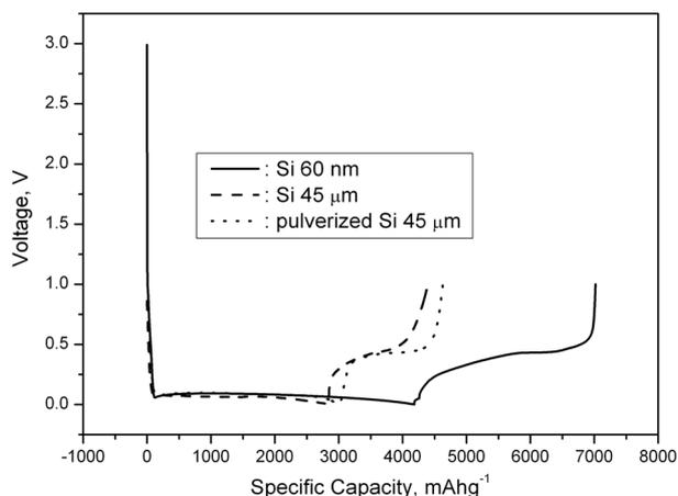
**Figure 1.** Voltage profiles of silicon anodes during the first cycle (current density: 0.25 mAcm<sup>-2</sup>).
