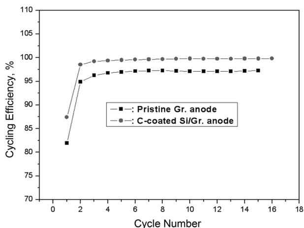
**Figure 7.** Cyclic efficiency of C-coated Si/Gr. anode and pristine Si/Gr. anode.
