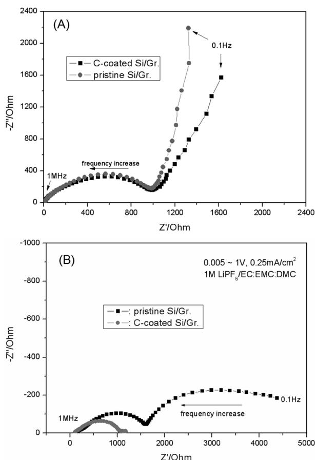
**Figure 4.** AC impedance spectrum of Li/Si cells before cycle test (A) and after 5<sup>th</sup> cycle test (B).
