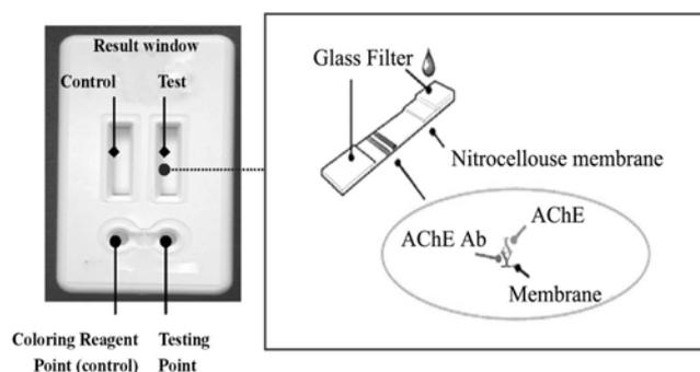
**Figure 1.** Composition of simple pesticide residue detection strip.
