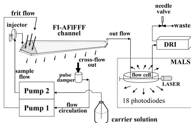
**Figure 1.** System configuration of the on-line frit-inlet asymmetrical flow field-flow fractionation/multiangle light scattering/differential refractive index detection (FI-AFIFFF/MALS/DRI). Field programming was achieved by circulating the cross-flow to frit flow.
