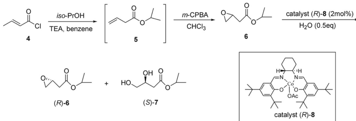
**Scheme 1.** Synthesis of chiral epoxide, (*R*)-**6**.
