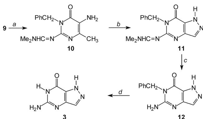
**Scheme 2.** (a) Pd/C, H<sub>2</sub> (60 psi), MeOH, rt; (b) NaNO<sub>2</sub>, AcOH, ~-10 °C, 3 h; (c) NH<sub>3</sub>/MeOH, rt, 3 h; (d) HCO<sub>2</sub>NH<sub>4</sub>, MeOH, Pd/C, reflux.
