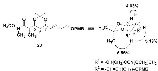
**Scheme 5.** Determination of relative stereochemistry of 1,3-*anti* acetonide **20**.
