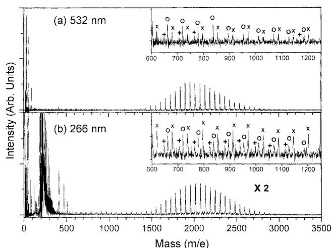
**Figure 1.** (a) Visible-SALDI and (b) UV-MALDI mass spectrum of PPG 2000 deposited on graphite plate using 532 nm and 266 nm laser radiation, respectively. In UV-MALDI, dithranol was used as a matrix. Symbols, x, + and o denoted in expanded insets represent  $58n+69$ ,  $58n+81$  and  $58n+97$  mass series of the fragment ion, respectively.
