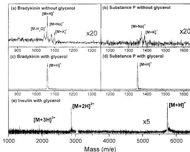
**Figure 5.** Visible SALDI mass spectra of bradykinin, substance P and insulin molecules. (a) and (b) were obtained using no any cationization agent and were smoothed to improve the signal-to-noise ratio. For (c), (d) and (e), glycerol was used as protonation agent.
