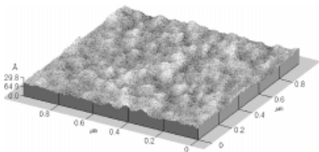
**Figure 3.** An AFM image of the Ga<sub>2</sub>O<sub>3</sub> film grown at 600 °C. The image was obtained over the area of 1 × 1 μm<sup>2</sup> in a non-contact mode.
