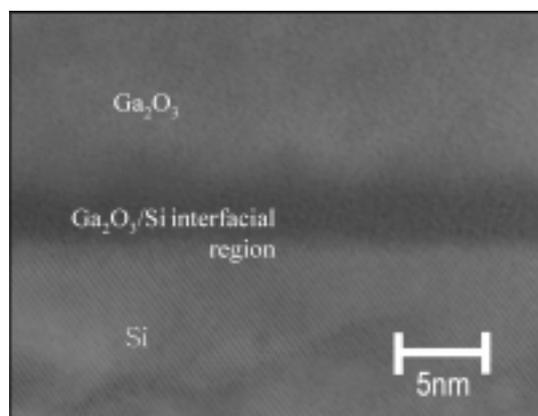
**Figure 4.** A cross-sectional TEM image of the Ga<sub>2</sub>O<sub>3</sub> film grown at 600 °C.
