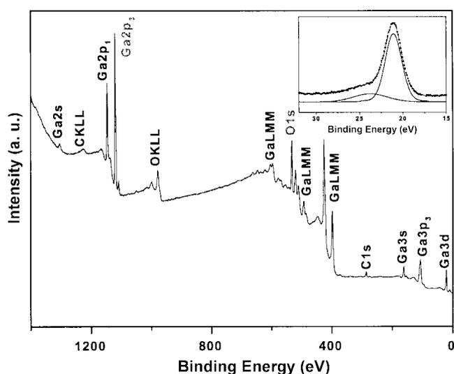
**Figure 1.** X-ray photoelectron survey spectrum of the gallium oxide thin film deposited at the substrate temperature of  $\sim$ 600 °C for 8 h. In the inset, the Ga 3d core level spectrum is shown with the curve-fitted results.
