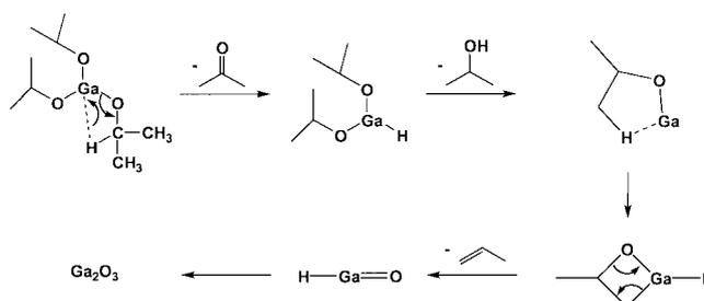
**Figure 5.** A proposed mechanism of the Ga<sub>2</sub>O<sub>3</sub> CVD using Ga(O<sup>*i*</sup>Pr)<sub>3</sub> as precursor.
