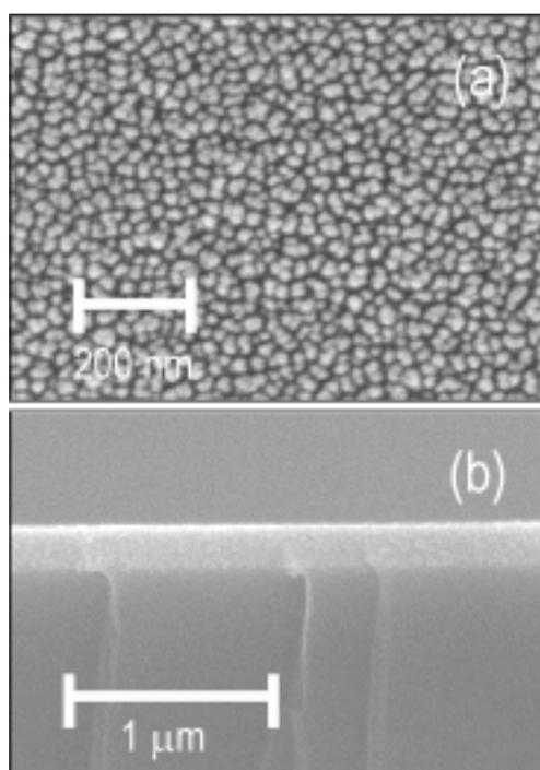
**Figure 2.** Plan-view (a) and cross-sectional (b) SEM images of the Ga<sub>2</sub>O<sub>3</sub> film of Figure 1.
