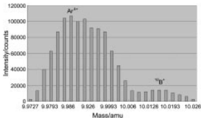
**Figure 1.** Mass spectrum showing slight overlapping of  $^{40}\text{Ar}^{4+}$  peak onto  $^{10}\text{B}^+$  peak.
