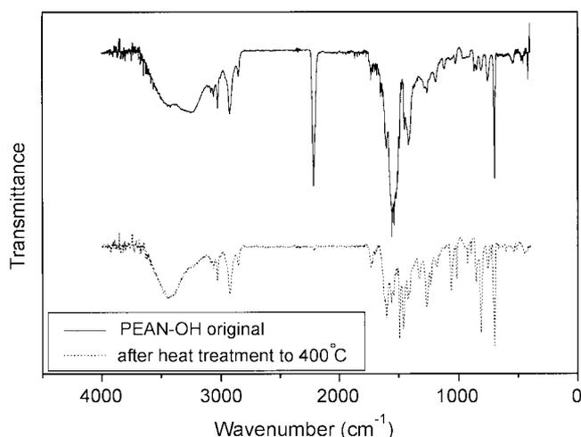
**Figure 6.** IR spectra of *o*-hydroxy polyenaminonitrile (VII); (a) before and (b) after curing reaction.
