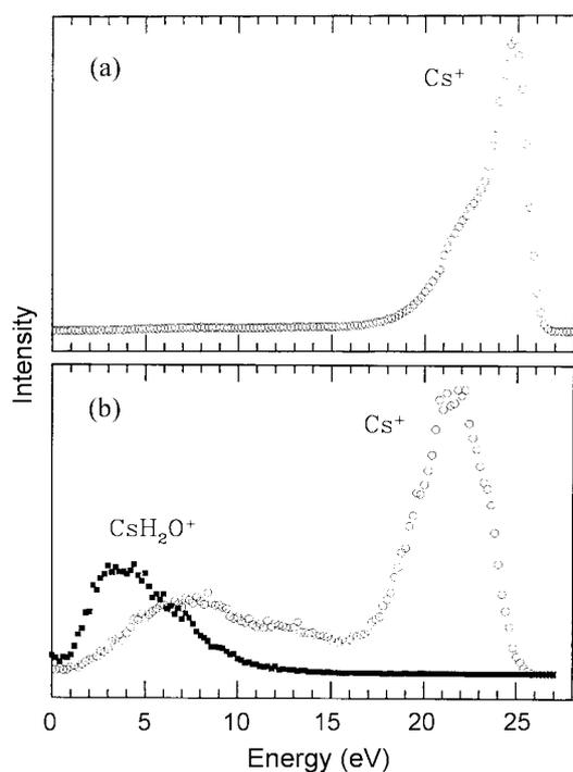
**Figure 5.** (a) Energy distribution of  $\text{Cs}^+$  ions scattered from a clean Pt(111) surface. (b) Energy distribution of  $\text{Cs}^+$  and  $\text{CsH}_2\text{O}^+$  scattered from a Pt(111) surface exposed to 0.75 L of  $\text{H}_2\text{O}$  at temperature of 100 K. The instrumental conditions were the same in (a) and (b):  $\text{Cs}^+$  beam energy was 30 eV, incident and exit angles were both  $70^\circ$  with respect to the surface plane (specular geometry).
