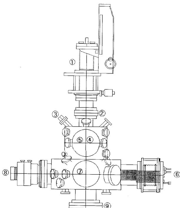
**Figure 1.** Overview of the angle-resolved reactive ion scattering chamber. The labeled components are: ① sample manipulator (x, y, z-motion), ② rotatable flange, ③ sputter ion gun, ④ view port, ⑤ CMA for AES (back side), ⑥ QMS, ⑦ view port, ⑧ TMP, ⑨ rotatable flange (ion gun stage).
