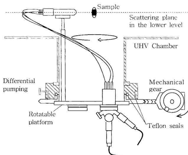
**Figure 3.**  $\text{Cs}^+$  ion gun mounted on a rotating flange. The ion gun rotates on a scattering plane defined by the positions of the gun, sample center, and QMS.
