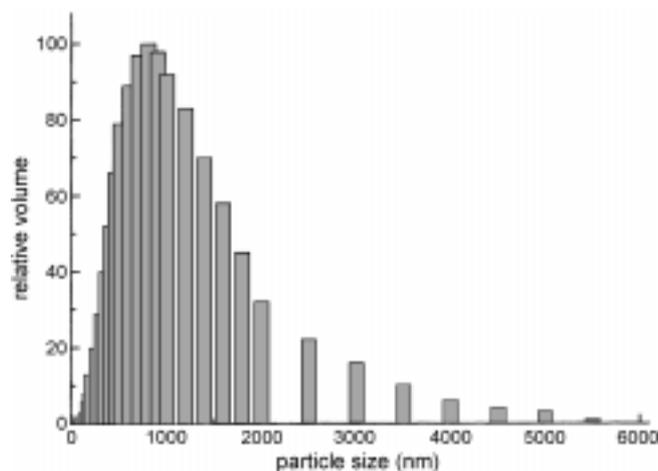
**Figure 1.** Particle size distribution of commercial Si<sub>3</sub>N<sub>4</sub> powder.
