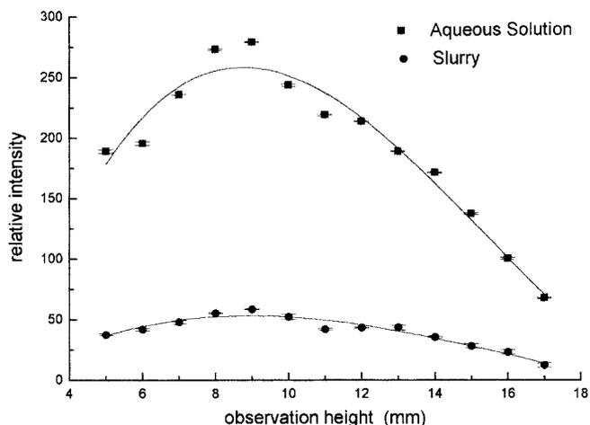
**Figure 3.** Intensity change of Fe (238.204 nm) for Si<sub>3</sub>N<sub>4</sub> slurry as the observation height varied in ICP-AES.
