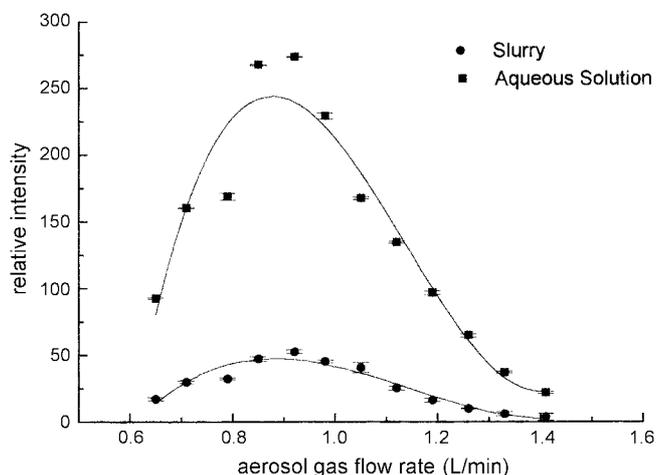
**Figure 4.** Influence of aerosol gas flow rate on Fe (230.204 nm) intensity for Si<sub>3</sub>N<sub>4</sub> slurry in ICP-AES.
