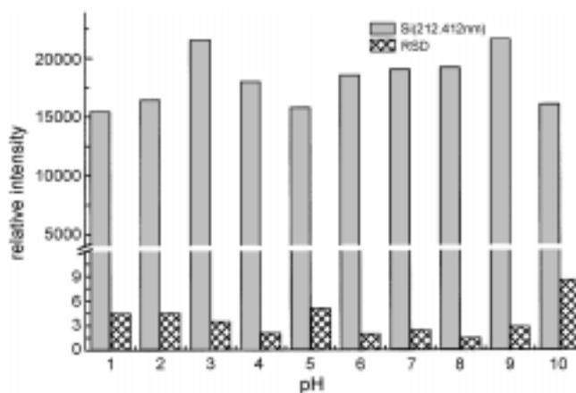
**Figure 2.** Effect of pH on the emission intensity of Si (212.412 nm) and its relative standard deviation in slurry injection ICP-AES.
