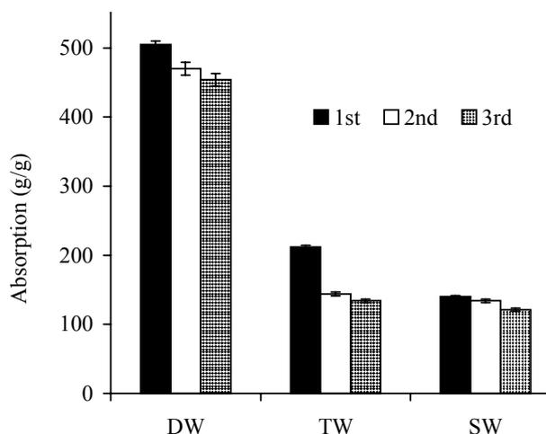
Figure 1. Absorption of distilled water (DW), tap water (TW) and saline water (SW) by gel during 1<sup>st</sup>, 2<sup>nd</sup> and 3<sup>rd</sup> wetting and drying cycle
