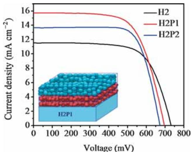
**Figure 8.** Photocurrent–voltage characteristics of DSCs with multilayer photoanodes of H2, H2P1 and H2P2.
