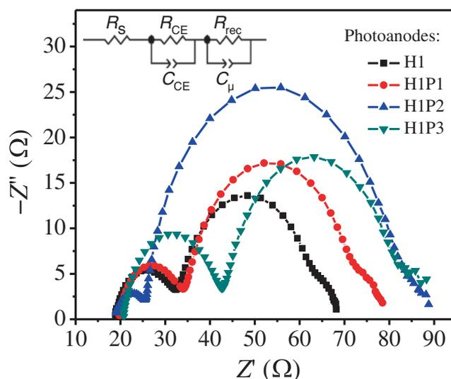
**Figure 7.** Nyquist plots of the dye-sensitized solar cells with H1, H1P1, H1P2 and H1P3 photoanodes measured at  $-0.8$  V in dark. The inset of the figure shows the equivalent circuit used for modelling of the impedance data.
