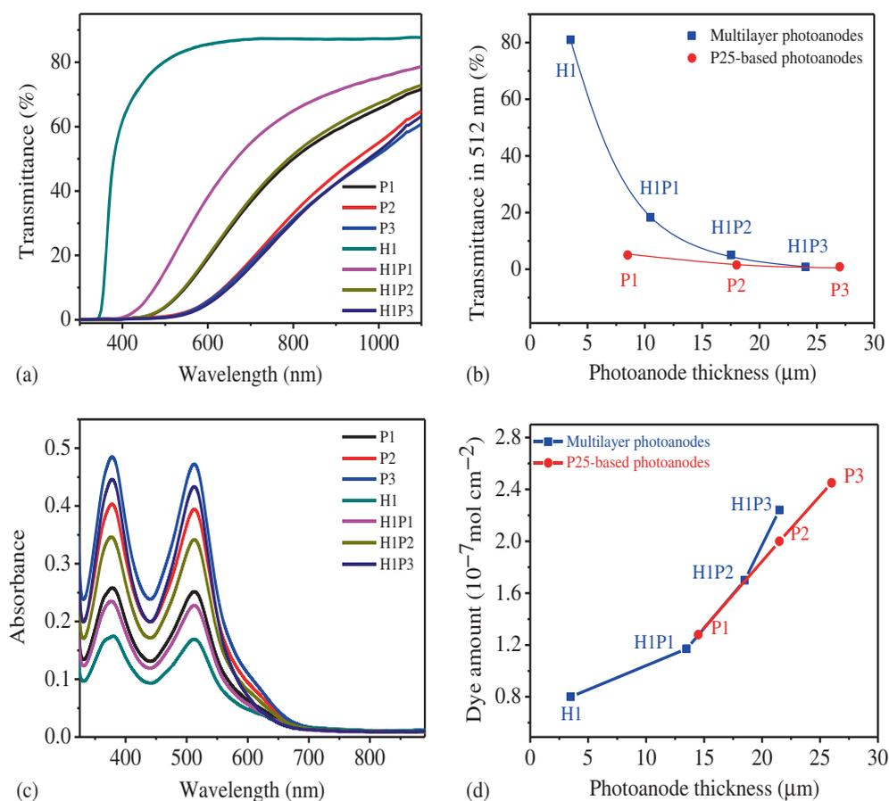
**Figure 5.** (a) Optical transmittance and its corresponding value in 512 nm vs. (b) the thickness for the P1, P2, P3, H1, H1P1, H1P2 and H1P3 photoelectrodes. (c) Absorbance of the dye N719 that is fully desorbed from the surface of the mentioned photoanodes and (d) calculated dye loading amount vs. the photoanode thickness. Dye desorption process is performed in 3 ml of 0.1 M NaOH solution in a mixed solvent of ethanol and water (water/ethanol = 1:1, v/v).
