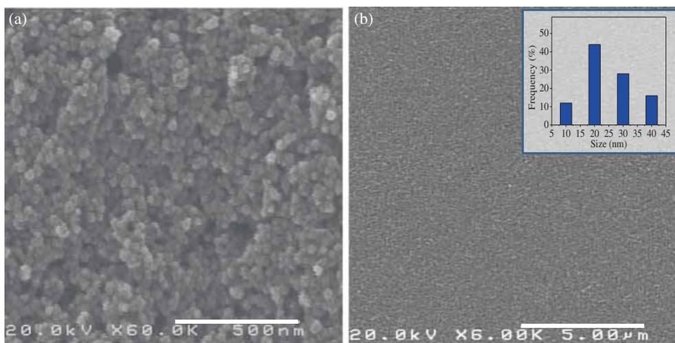
**Figure 2.** (a, b) SEM images of the hydrothermally grown TiO<sub>2</sub> nanocrystals in two different magnifications. The size distribution histogram of the nanocrystals is represented in the inset of b.
