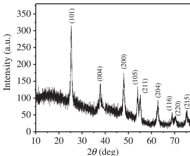
**Figure 3.** X-ray diffraction pattern of the hydrothermally grown TiO<sub>2</sub> nanocrystals.
