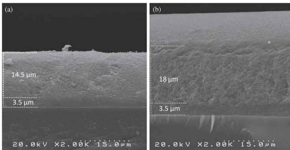
**Figure 4.** Cross-sectional SEM images of (a) HIP2 and (b) HIP3 multilayer photoanodes.
