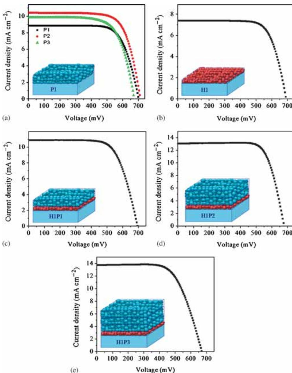
**Figure 6.** (a–e) Photocurrent–voltage ( $I$ – $V$ ) characteristics of the dye-sensitized solar cells with H1, P1, P2, P3, H1P1, H1P2 and H1P3 photoelectrodes.
