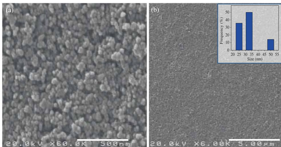
**Figure 1.** (a, b) SEM images of the P1 layer composed of P25  $\text{TiO}_2$  nanocrystals in two different magnifications. The size distribution histogram of the particles is shown in inset of **b**.
