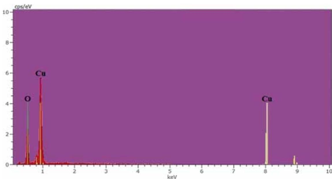
**Figure 5.** EDX pattern of *Eichhornia*-mediated copper oxide nanoparticles.
