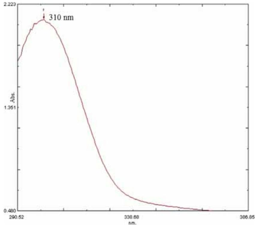
**Figure 2.** UV spectra of *Eichhornia*-mediated copper oxide nanoparticles.
