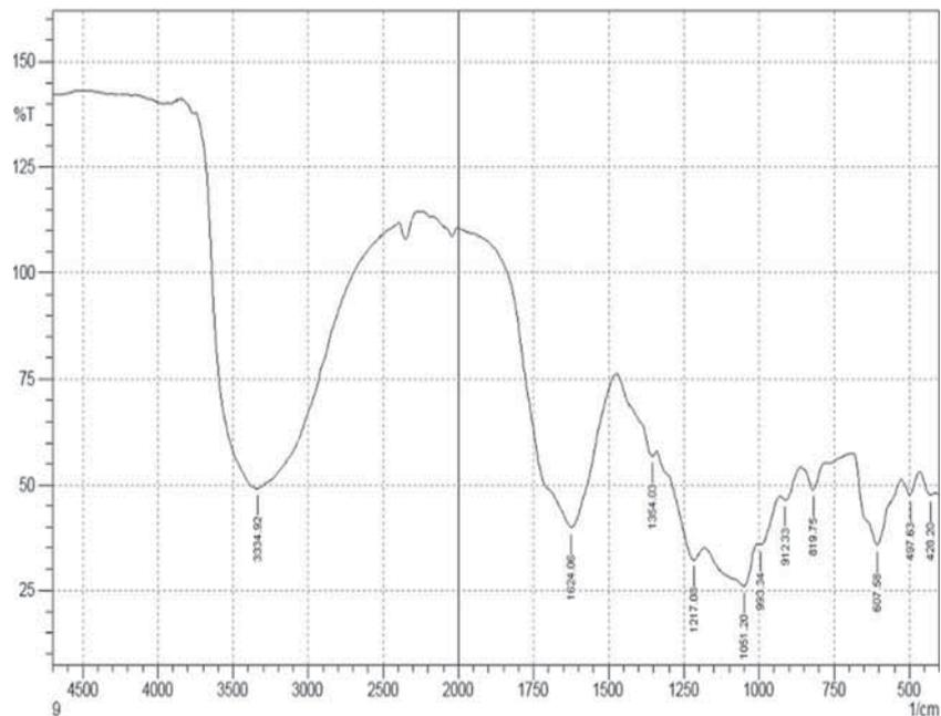
**Figure 3.** FTIR spectra of *Eichhornia* copper oxide nanoparticles.
