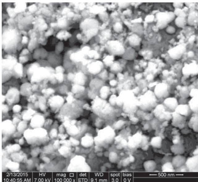
**Figure 4.** FESEM image of *Eichhornia*-mediated copper oxide nanoparticles.
