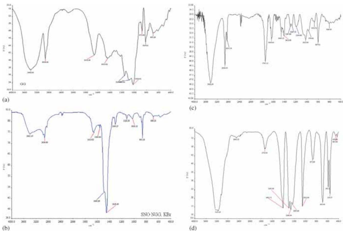
**Figure 1.** FT-IR spectra of (a) guar-gum (GG), (b) sodium salt of guar-gum (NaGG), (c) acrylated guar-gum (GG-AC) and (d) acrylic acid grafted on acrylated guar-gum (AA-GG-AC).
