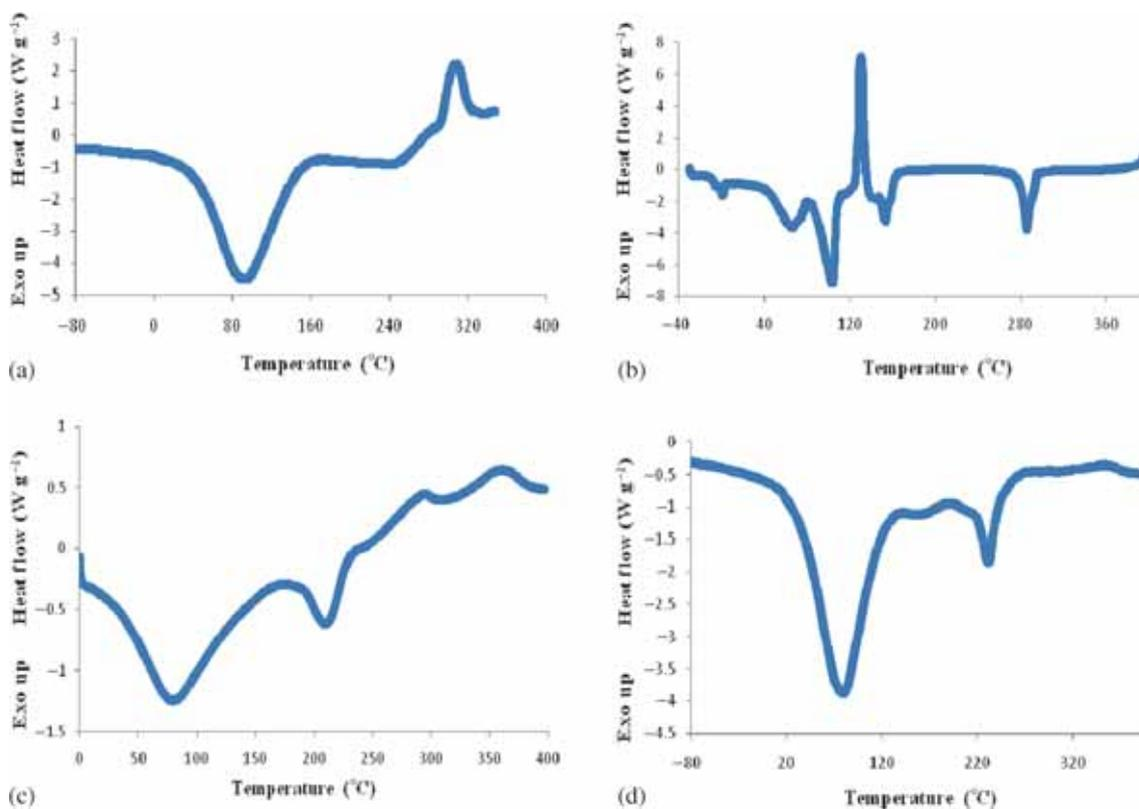
**Figure 2.** DSC thermogram of (a) pure guar-gum, (b) sodium salt of guar-gum, (c) acrylated guar-gum and (d) acrylic acid grafted guar-gum.
