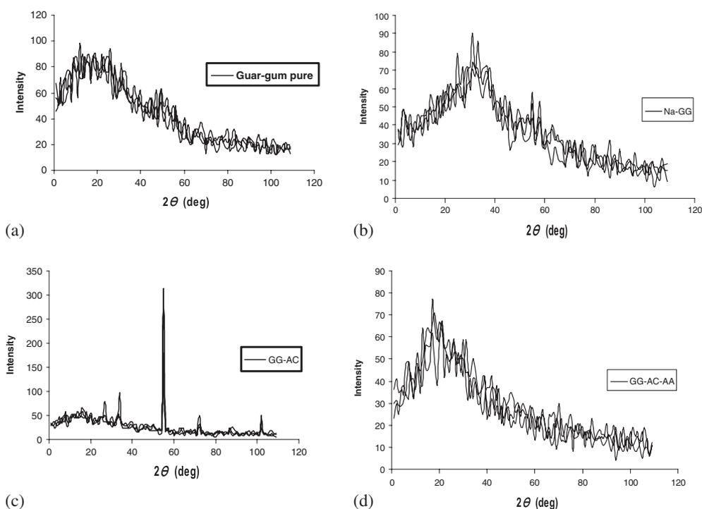
**Figure 3.** X-ray diffraction of (a) pure guar-gum, (b) sodium salt of guar-gum, (c) acrylated guar-gum and (d) acrylic acid grafted guar-gum product.
