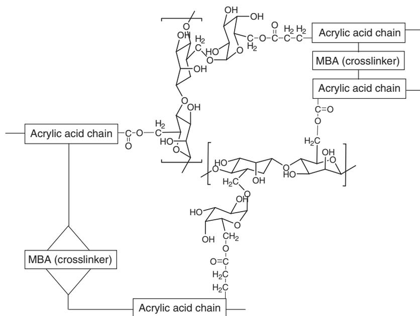
**Scheme 3.** Grafting of acrylic acid onto the acrylated guar-gum chain.
