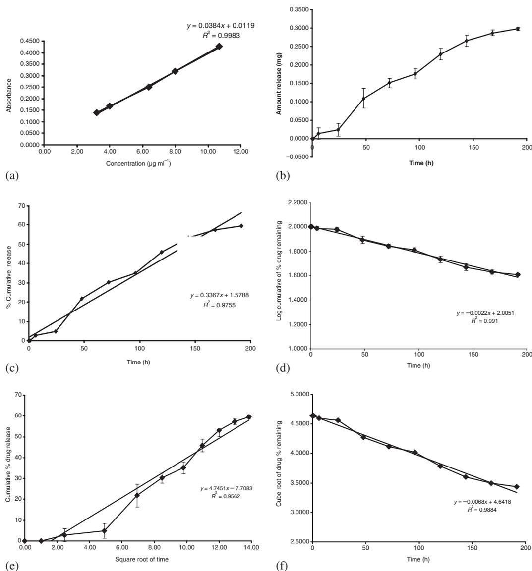
**Figure 4.** Standard curve of chlorpyrifos at  $\lambda_{228}$  nm in (a) methanolic buffer pH 7.4 (25:75 v/v%), (b) cumulative % chlorpyrifos release in various media, (c) zero-order release in methanolic buffer pH 7.4, (d) first-order release in methanolic buffer pH 7.4, (e) Higuchi release in methanolic buffer pH 7.4 and (f) Hixson–Crowell release methanolic buffer pH 7.4.
