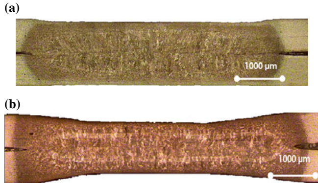
Figure 4. Microstructure photographs of specimens welded at different parameters: (a) DP450U, 3kA-10c and (b) DP450U, 9kA-40c.
