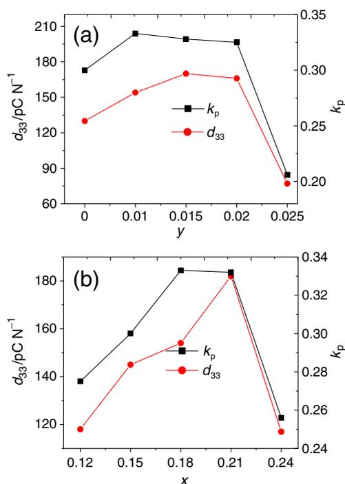
**Figure 4.** Piezoelectric constant,  $d_{33}$  and planar electromechanical coupling factor  $k_p$  of  $(1-x-y)\text{BNT}-x\text{BKT}-y\text{BM}$  ceramics: (a)  $x = 0.18$  and (b)  $y = 0.01$ .
