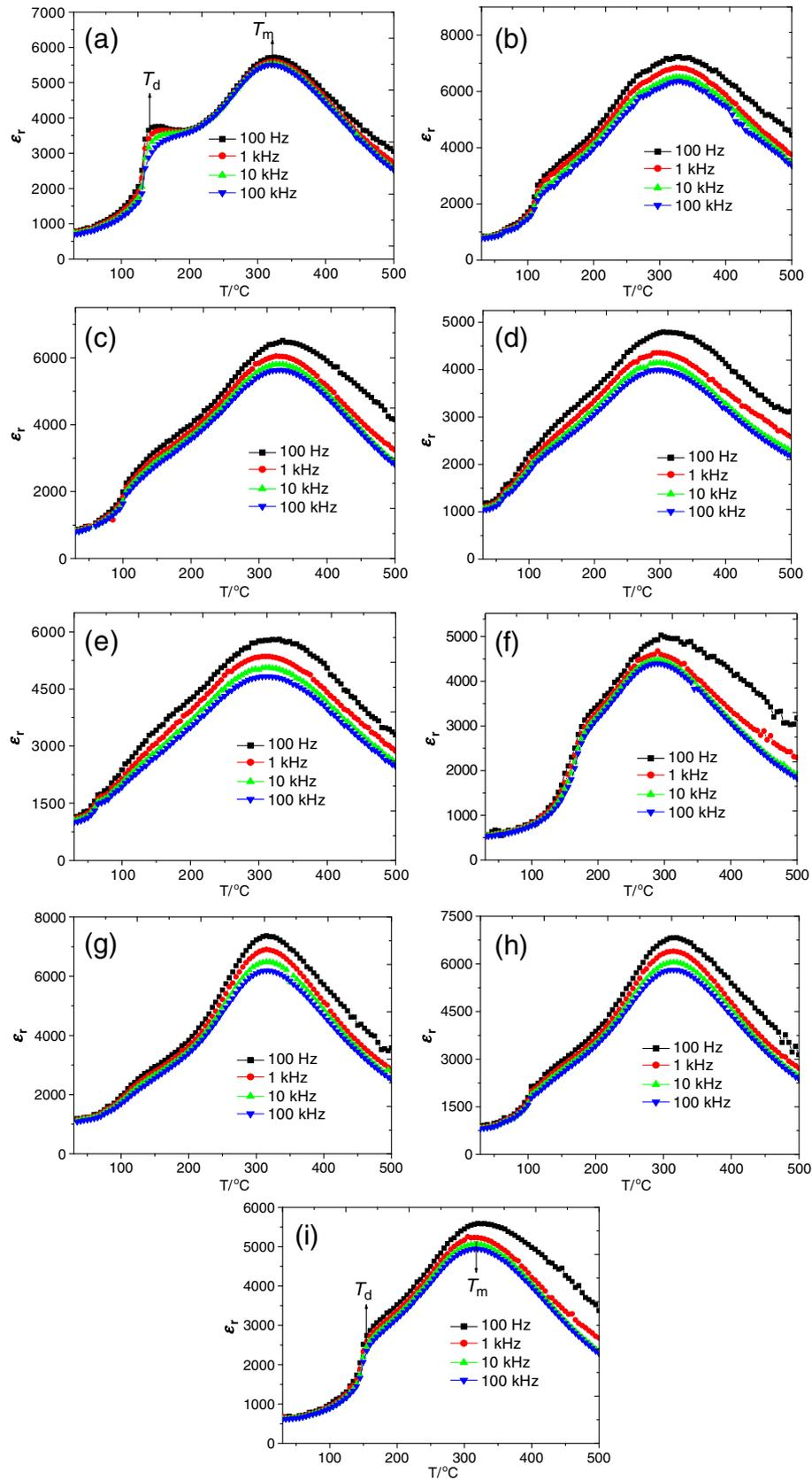
**Figure 3.** Temperature dependences of  $\epsilon_r$  for poled  $(1-x-y)\text{BNT}-x\text{BKT}-y\text{BM}$  samples: (a)  $x = 0.18$ ,  $y = 0$ ; (b)  $x = 0.18$ ,  $y = 0.01$ ; (c)  $x = 0.18$ ,  $y = 0.015$ ; (d)  $x = 0.18$ ,  $y = 0.02$ ; (e)  $x = 0.18$ ,  $y = 0.025$ ; (f)  $x = 0.12$ ,  $y = 0.01$ ; (g)  $x = 0.15$ ,  $y = 0.01$ ; (h)  $x = 0.21$ ,  $y = 0.01$  and (i)  $x = 0.24$ ,  $y = 0.01$ .
