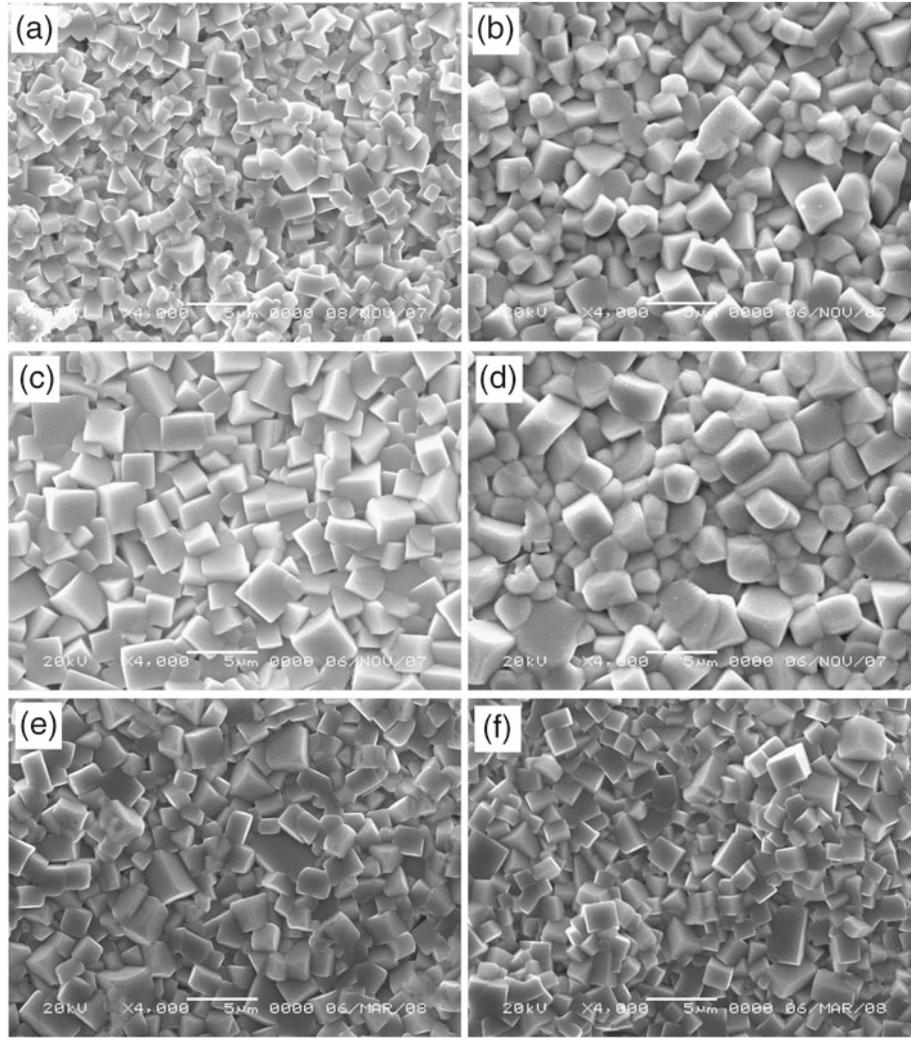
**Figure 2.** SEM images of  $(1 - x - y)\text{BNT}-x\text{BKT}-y\text{BM}$  ceramics: (a)  $x = 0.18$ ,  $y = 0$ ; (b)  $x = 0.18$ ,  $y = 0.01$ ; (c)  $x = 0.18$ ,  $y = 0.02$ ; (d)  $x = 0.18$ ,  $y = 0.025$ ; (e)  $x = 0.21$ ,  $y = 0.01$  and (f)  $x = 0.24$ ,  $y = 0.01$ .
