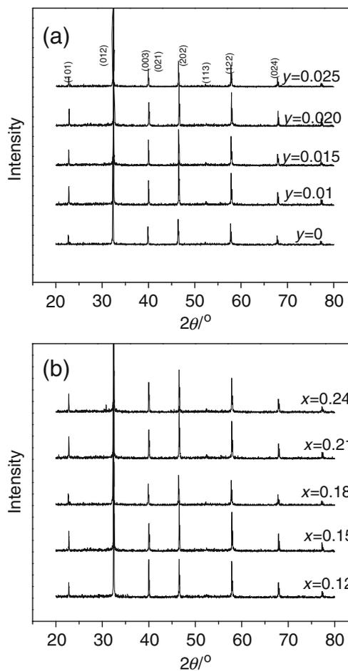
**Figure 1.** XRD pattern of  $(1-x-y)\text{BNT-}x\text{BKT-}y\text{BM}$  ceramics: (a)  $x = 0.18$  and (b)  $y = 0.01$ .
