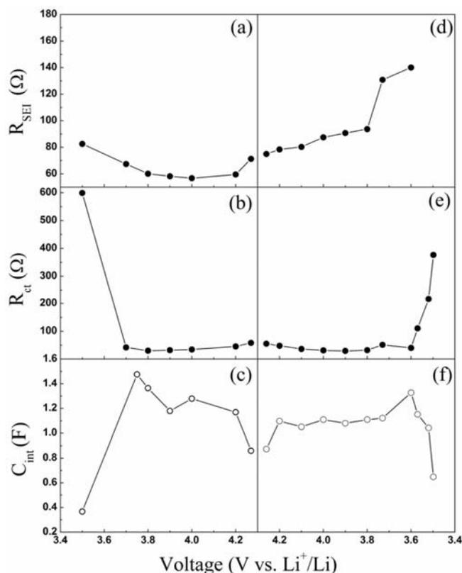
**Figure 8.** Variation in resistive and capacitive components for cell during lithium de-intercalation (a–c) and intercalation (d–f). Resistance due to SEI layer is denoted as  $R_{\text{SEI}}$  (a, d) and charge transfer resistance as  $R_{\text{ct}}$  (b, e).
