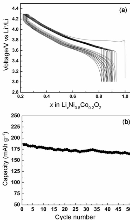
**Figure 4.** (a) Voltage vs composition data derived from galvanostatic charge/discharge experiments on  $\text{LiNi}_{0.8}\text{Co}_{0.2}\text{O}_2/\text{Li}$  cell in voltage range between 3 and 4.3 V at 0.2C rate and (b) discharge capacity vs cycle number.
