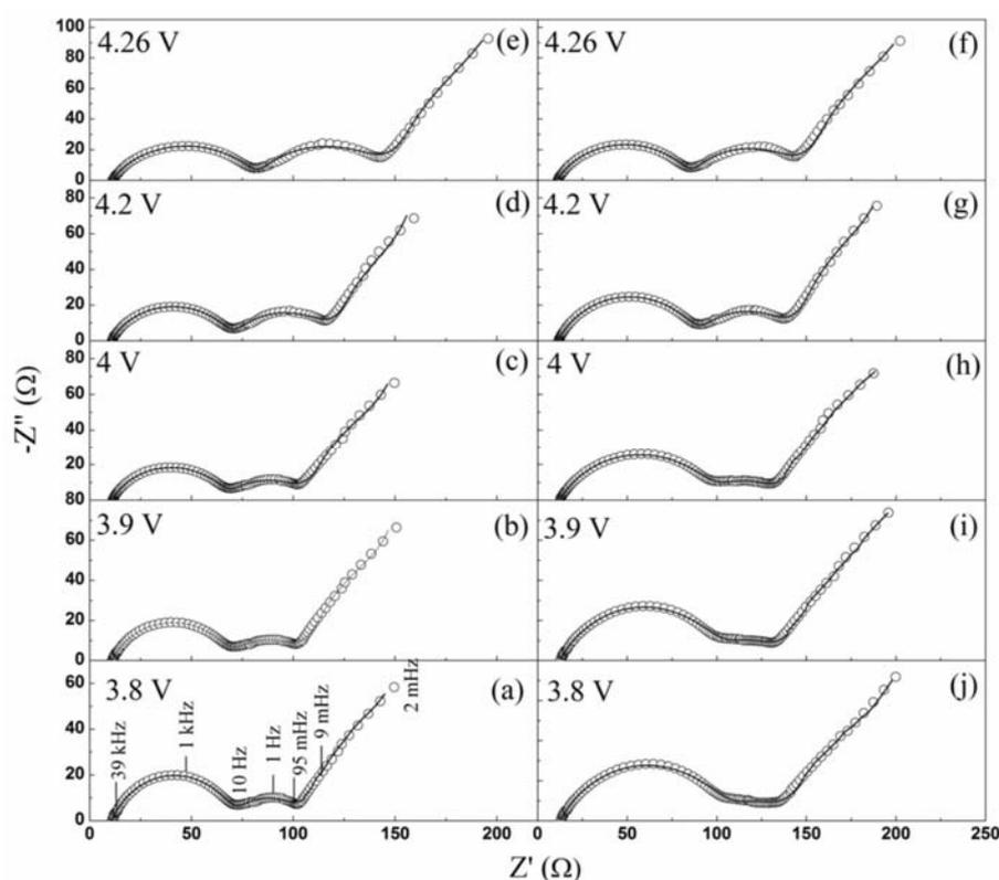
**Figure 6.** Nyquist plots for  $\text{LiNi}_{0.8}\text{Co}_{0.2}\text{O}_2$  half cells during de-intercalation (a–e) and intercalation (f–j) of lithium.
