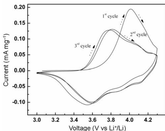
**Figure 3.** Cyclic voltammograms for  $\text{LiNi}_{0.8}\text{Co}_{0.2}\text{O}_2$  vs Li cells in voltage range 3–4.3 V with a scan rate of 0.1 mV/s.
