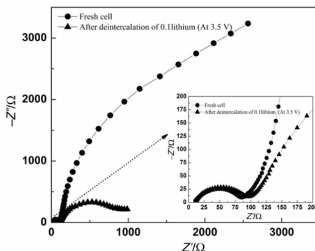
**Figure 5.** Impedance spectra for fresh cell together with that after de-intercalation of 0.1 Li in frequency range between 400 kHz and 2 mHz in galvanostatic mode. Inset shows magnified high-frequency region.
