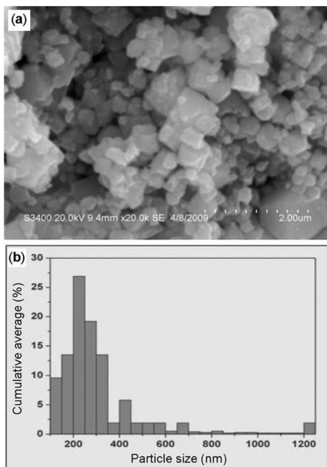
**Figure 2.** (a) Scanning electron micrograph for  $\text{LiNi}_{0.8}\text{Co}_{0.2}\text{O}_2$  and (b) histogram shows particle-size distribution.
