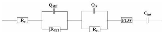
**Figure 7.** Equivalent circuit model used for fitting impedance spectrum.  $R_e$  is the ohmic resistance due to electrolyte,  $R_{\text{SEI}}$  and  $R_{\text{ct}}$  are total resistance associated with solid electrolyte interface and charge transfer, respectively.  $Q_{\text{SEI}}$  and  $Q_{\text{ct}}$  are constant phase elements for SEI and charge transfer. FLW is finite-length Warburg and  $C_{\text{int}}$  represents intercalative capacitance.
