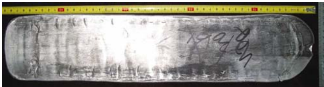
Figure 3. Appearances of Al/Mg/Al laminated composite fabricated by hot rolling.
