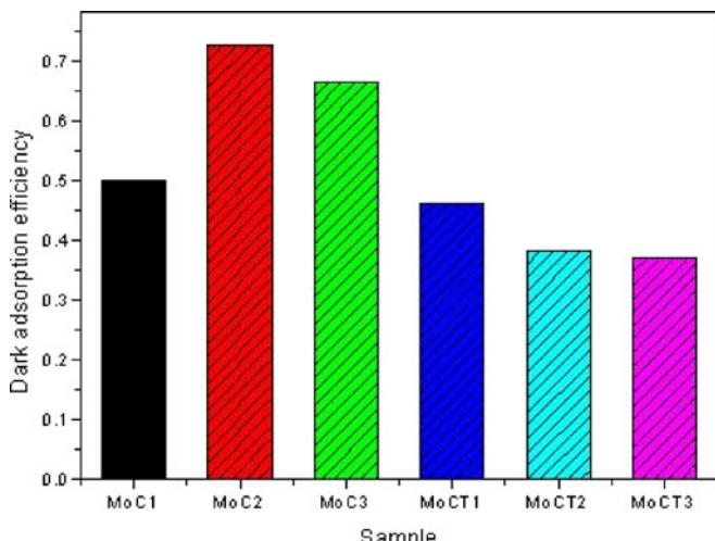
**Figure 5.** Dark adsorption efficiency of MoC and MoCT composites for MB degradation.
