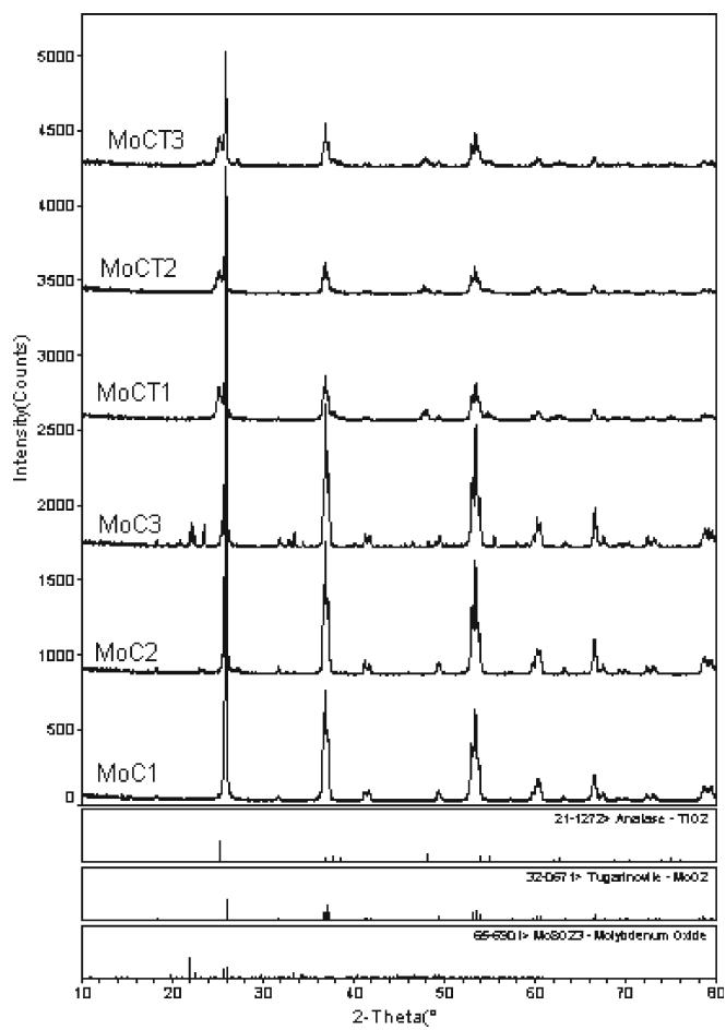
**Figure 2.** XRD patterns of Mo-CNT/TiO<sub>2</sub> composites.
