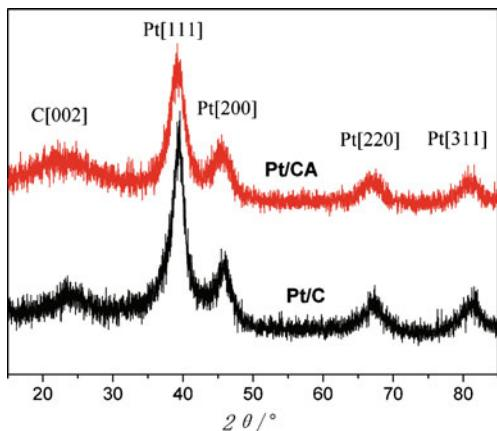
**Figure 2.** XRD patterns of Pt/CA catalyst and Pt/C catalyst (JM).
