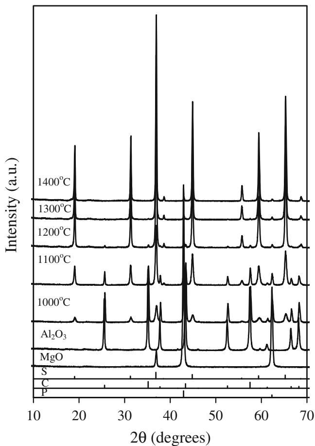
**Figure 3.** XRD patterns of as purchased  $\alpha$ - $Al_2O_3$  and calcined caustic  $MgO$ , and of the  $MgAl_2O_4$  spinel powders formed upon calcination for 1 h at temperatures between 1000 and 1400°C. P, periclase, ICDD File No: 00–45–946; C, corundum, ICDD File No: 00–46–1212; S, spinel, ICDD File No: 00–21–1152.
