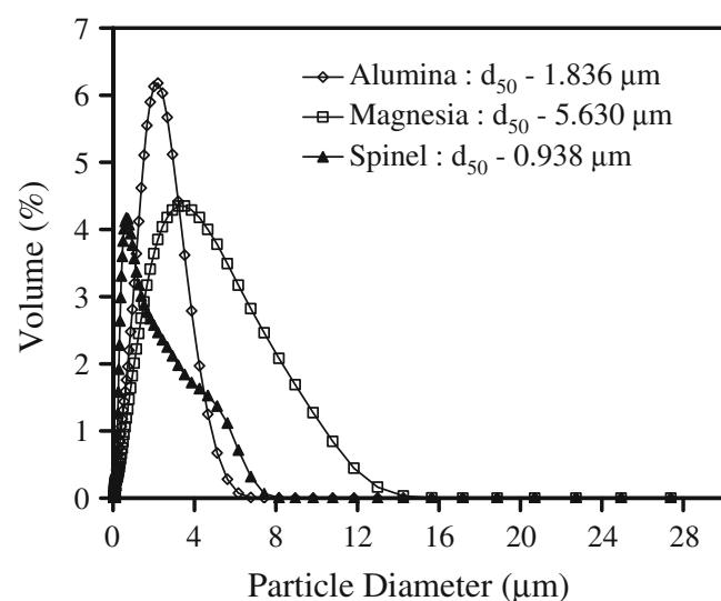
Figure 2. Particle size distributions of as purchased  $\alpha\text{-Al}_2\text{O}_3$  and calcined caustic  $\text{MgO}$  powders, and of the planetary ball milled  $\text{MgAl}_2\text{O}_4$  spinel formed at  $1400^{\circ}\text{C}$  for 1 h.
