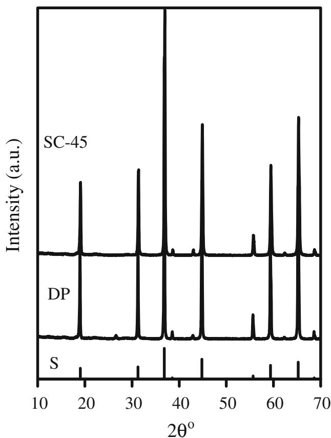
**Figure 6.** XRD patterns of DP and SC-45 consolidated bodies sintered for 1 h at 1650°C and 2 h at 1600°C, respectively. S, spinel, ICDD File No. 00-21-1152.
