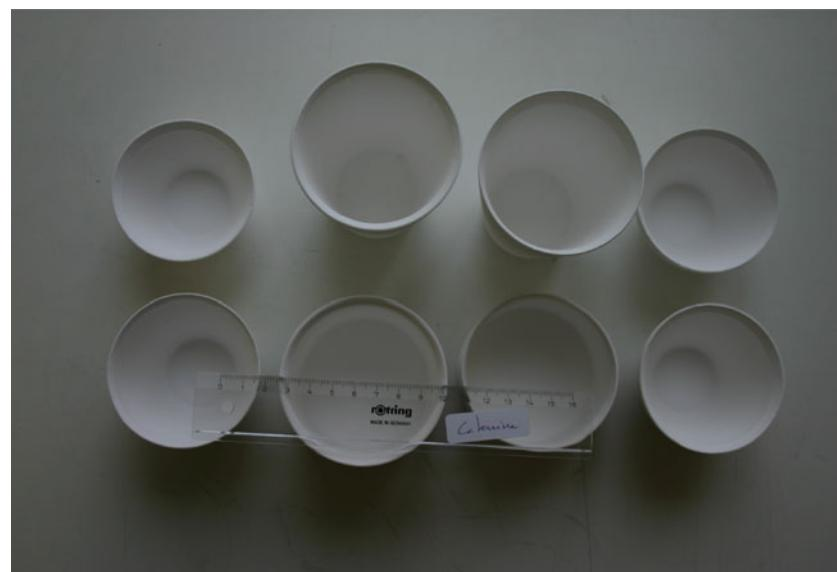
**Figure 1.** Green  $MgAl_2O_4$  spinel crucibles consolidated by aqueous slip casting from a suspension containing 45 vol.% solids loading.
