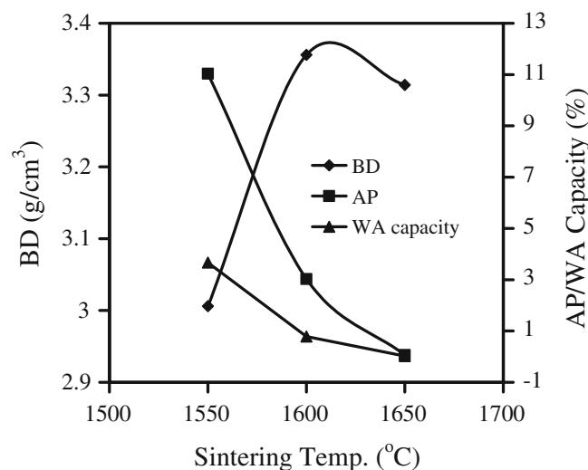
**Figure 5.** Evolution of bulk density (BD), apparent porosity (AP) and water absorption (WA) capacity of  $MgAl_2O_4$  spinel consolidated by slip casting route using aqueous suspension containing 45 vol.% solids and sintered for 2 h at 1550–1650°C.
