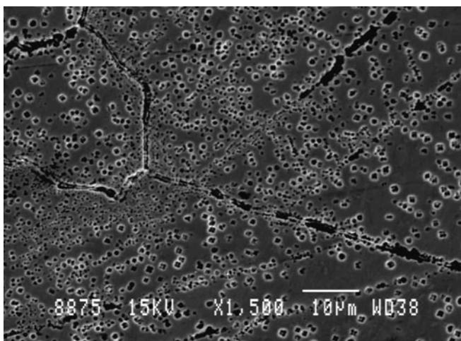
**Figure 1.** SEM microstructure of sample aged at 1073 K for 50 h showing extensive precipitation of coherent  $\gamma'$  intermetallic phase.
