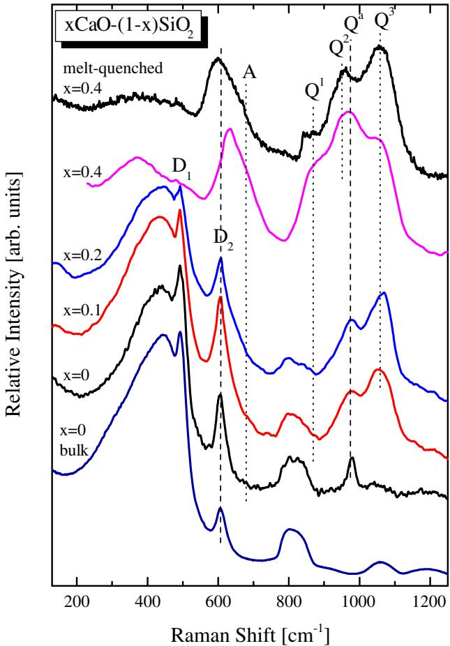
**Figure 2.** Representative Stokes-side Raman spectra of  $x\text{CaO}\cdot(1-x)\text{SiO}_2$  ( $x = 0, 0.1, 0.2$  and  $0.4$ ) glasses prepared by sol-gel technique at room temperature. The Raman spectra of the bulk, melt-quenched  $\text{SiO}_2$  and the  $0.4\text{CaO}\cdot0.6\text{SiO}_2$  glasses are also shown at the bottom and top of this figure, respectively.
