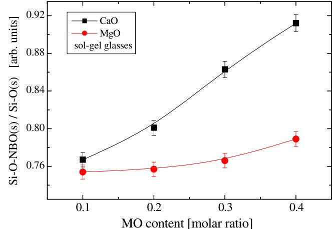
**Figure 4.**  $\text{Si}-\text{O}-\text{NBO}(s)/\text{Si}-\text{O}(s)$  absorbance intensity ratio versus modifier composition for the  $x\text{MO}\cdot(1-x)\text{SiO}_2$  ( $\text{M} = \text{Ca}, \text{Mg}$ ) glasses. Lines are drawn as guide to the eye.
