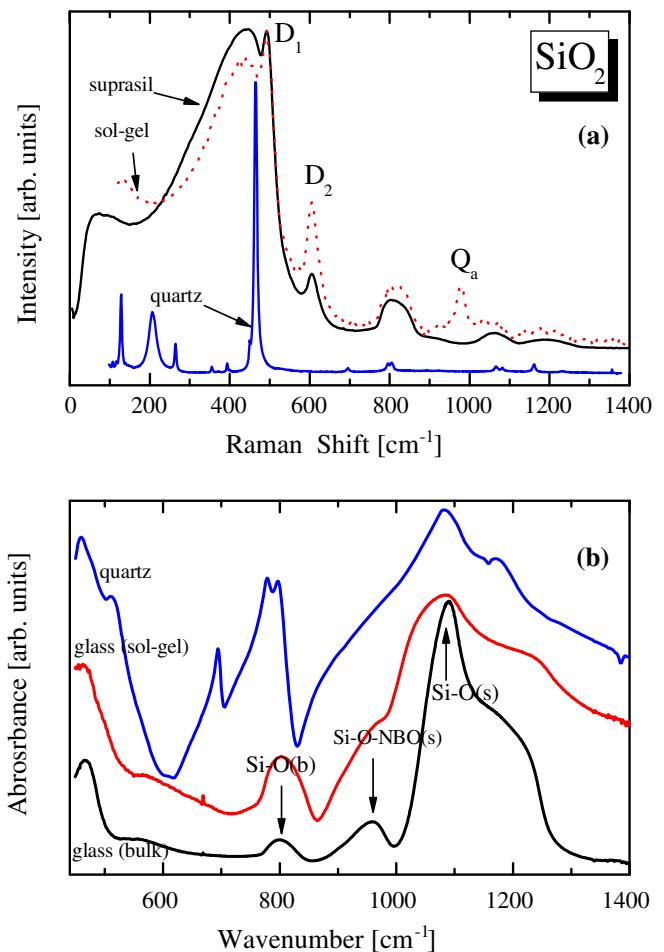
**Figure 1.** Raman spectra (a) and IR absorbance spectra (b) of pure melt-quenched and sol-gel derived silica glass. The Raman and IR spectra of quartz crystal are also shown for comparison.
