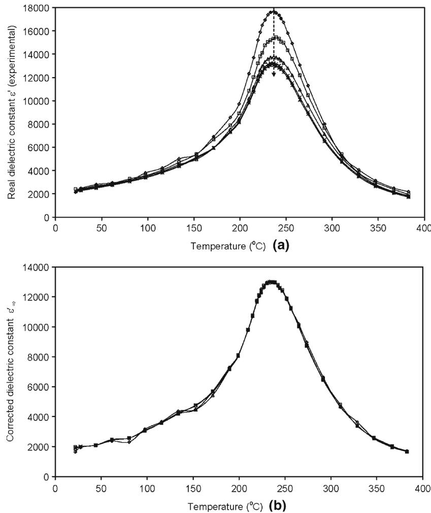
**Figure 3.** Behaviour of the real part of the dielectric constant with temperature: (a) experimental data of dielectric constant corresponding to 1, 10, 100, 1000 and 10000 Hz, and (b) corrected data of dielectric constant at same frequencies. Arrow in 3(a) indicates the increasing direction of frequency at peak dielectric constant value. The data presented in this figure corresponds to  $x = 6.0$  at% of La.
