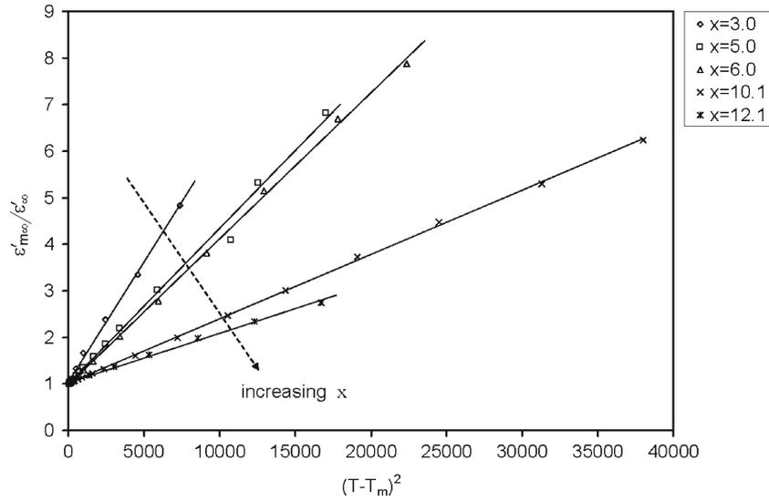
**Figure 9.** Variation of normalized dielectric constant,  $\varepsilon'_{m\infty}/\varepsilon'_{\infty}$ , in paraelectric region vs square of normalized temperature for all compositions. The solid straight lines are the linear fits for the corresponding data. The arrow indicates increasing direction of La concentration in base PZT.
