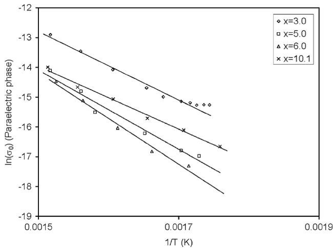
**Figure 6.** Arrhenius plot of d.c. conductivity in the paraelectric region for different compositions. The d.c. conductivity is determined from fitting of imaginary part of dielectric data in paraelectric region. It is very difficult to estimate the value of d.c. conductivity in ferroelectric region as d.c. conductivity is very low and also dispersion phenomenon starts at low frequency below transition region and spreads in several decades around peak frequency corresponding to  $\epsilon''$ .
