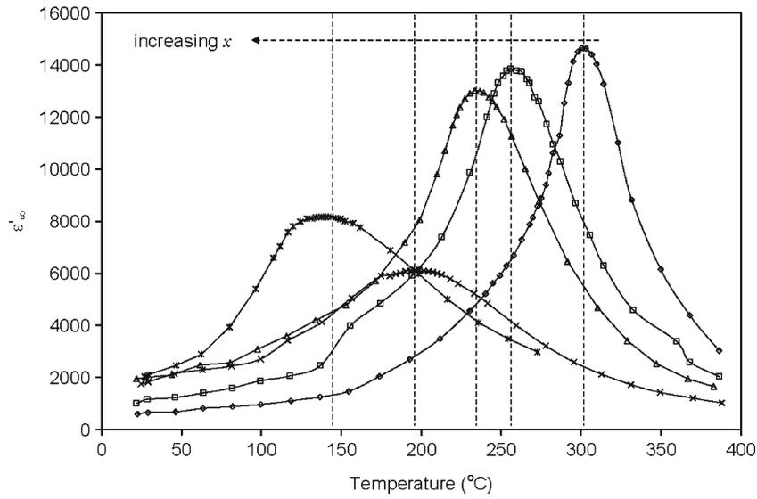
**Figure 4.** Change in the high frequency limiting value of the dielectric constant,  $\epsilon'_{\infty}$ , with temperature corresponding to different samples of PLZT. These values are determined from fitting of dielectric data in both non-dispersive and dispersive regions. The vertical lines correspond to the maximum dielectric constant with temperature,  $T_m$ , for respective compositions.
