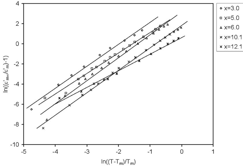
**Figure 10.** Plot of  $\ln((\varepsilon'_{m\infty}/\varepsilon'_m) - 1)$  vs  $\ln((T - T_m)/T_m)$  in paraelectric region for various compositions of PLZT.
