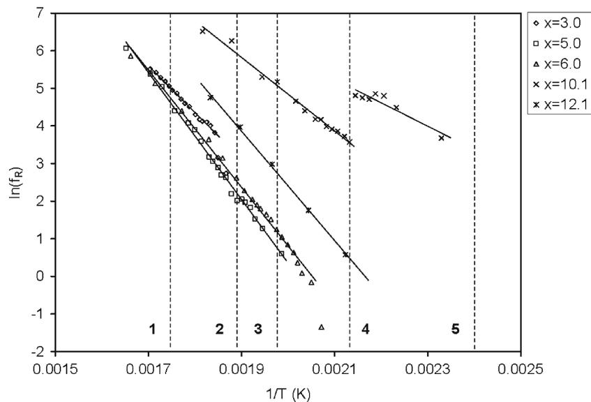
**Figure 5.** Arrhenius behaviour of relaxation frequency corresponding to different compositions. Vertical dotted lines 1, 2, 3, 4 and 5 represent the transition temperature,  $T_m$ , with increasing concentration, respectively.
