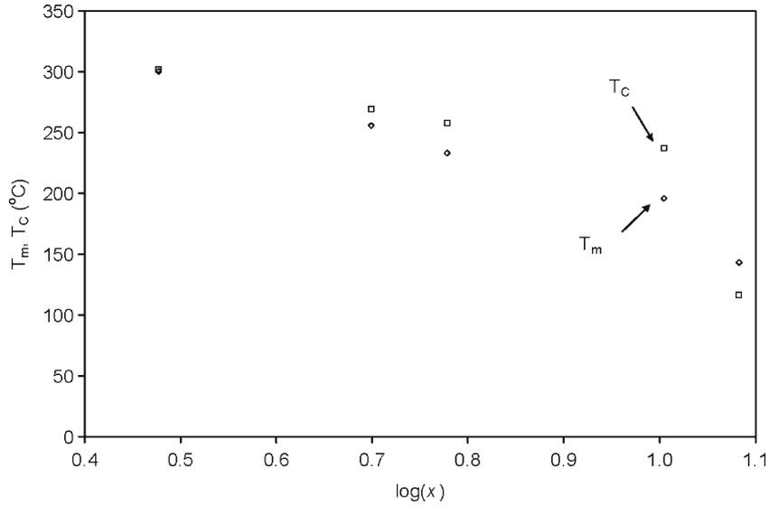
**Figure 8.** Concentration dependence of  $T_m$  and extrapolated Curie temperature,  $T_c$ , for La-doped PZT.
