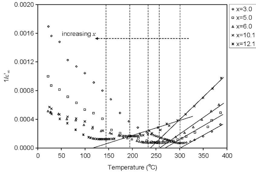
**Figure 7.** Variation of inverse of the  $\varepsilon'_{\infty}$  with temperature for each composition. The dotted vertical lines show the transition temperature for each composition from right to left respectively which is indicated by arrow in the figure. The solid lines are the linear fits to corresponding data in paraelectric region. Arrow indicates the direction of increasing concentration of La in base PZT.
