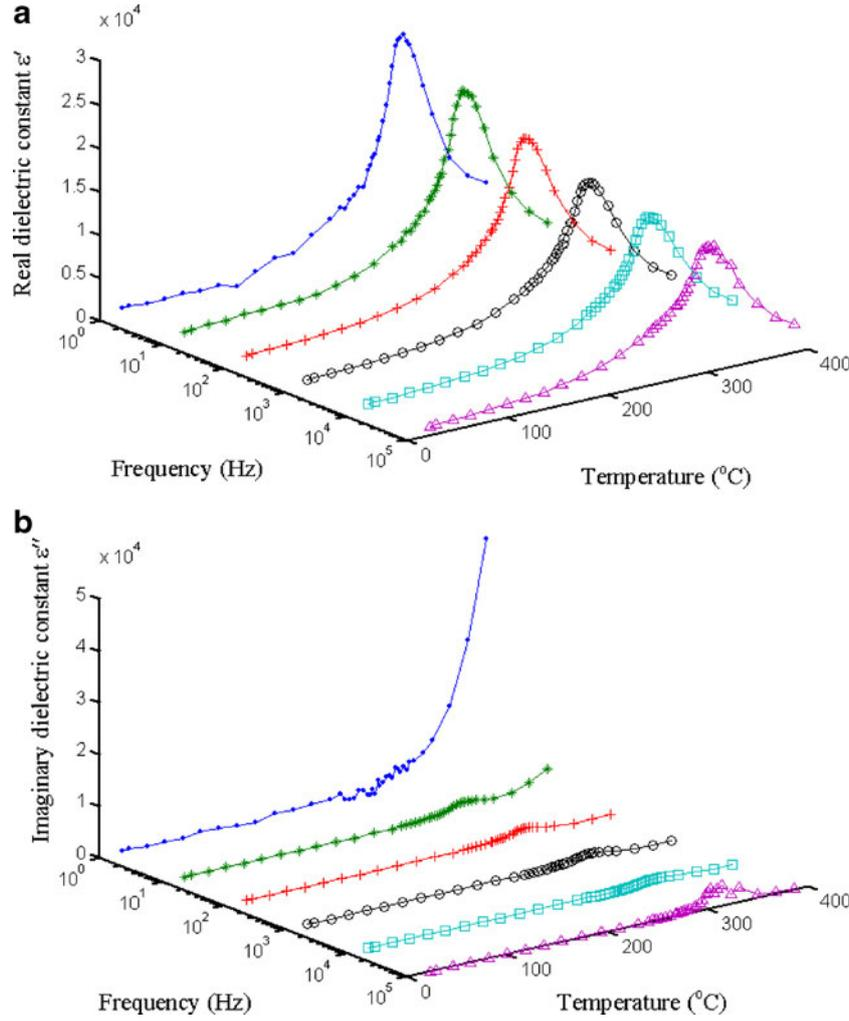
**Figure 1.** Variation of the real and imaginary parts of the dielectric constant with temperature at selected frequencies for  $x = 3.0$  at% of La.
