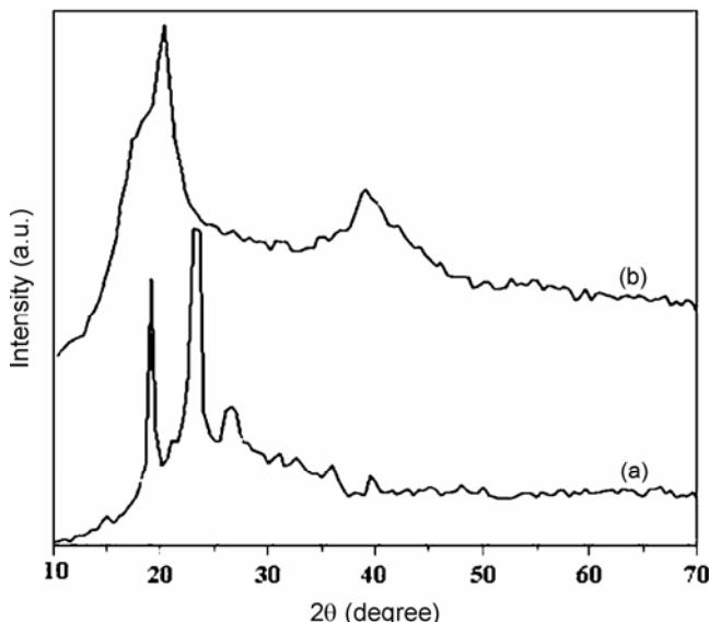
**Figure 7.** XRD spectra of (a) PEO and (b) P(VdF-HFP).
