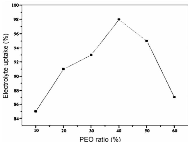
**Figure 3.** Liquid electrolyte uptake of P(VdF-HFP)-x% PEO microporous membranes as a function of PEO weight ratio.
