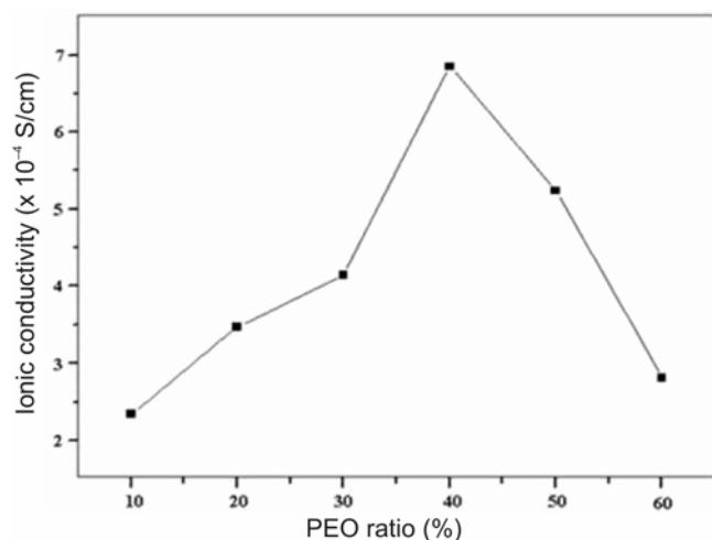
**Figure 5.** Ionic conductivity of P(VdF-HFP)-x% PEO microporous membranes as a function of PEO weight ratio.
