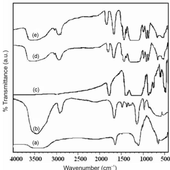
**Figure 9.** FTIR spectra of (a) LiClO<sub>4</sub>, (b) pure PEO, (c) pure P(VdF-HFP), (d) P(VdF-HFP)-30% PEO and (e) P(VdF-HFP)-50% PEO.
