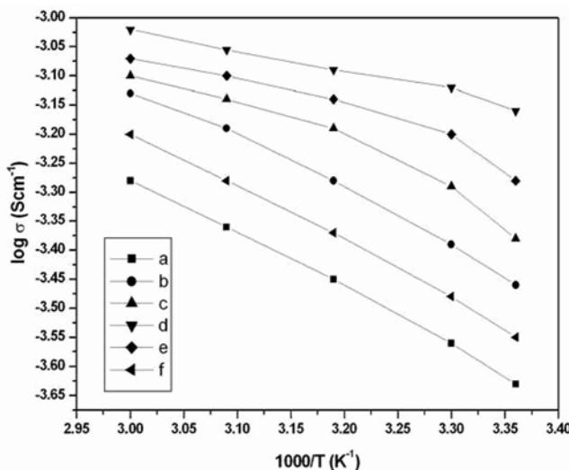
**Figure 6.** Temperature dependence of ionic conductivity of P(VdF-HFP)- $x\%$  PEO microporous polymer electrolytes: (a)  $x = 10$ ; (b)  $x = 20$ ; (c)  $x = 30$ ; (d)  $x = 40$ ; (e)  $x = 50$  and (f)  $x = 60$ .
