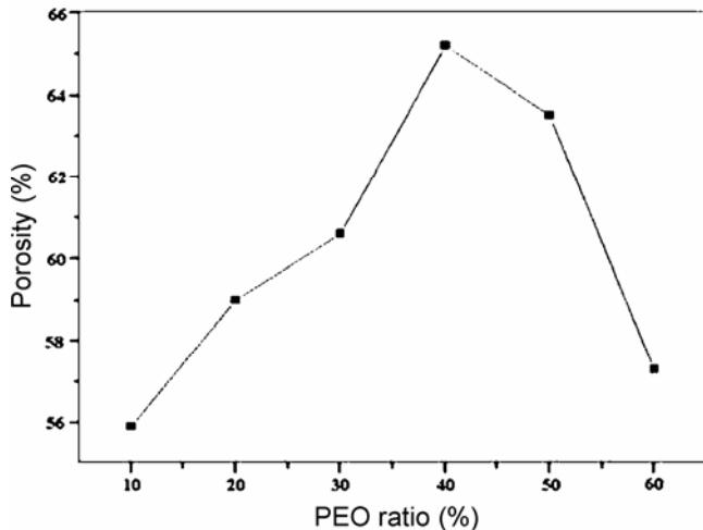
**Figure 2.** Porosity of P(VdF-HFP)-x% PEO microporous membranes as a function of PEO weight ratio.
