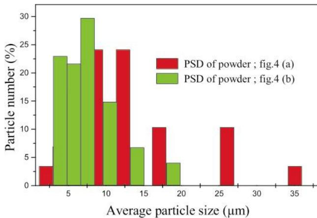
**Figure 4.** Histograms of powders before and after compaction.
