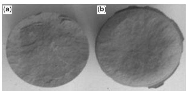
**Figure 2.** Fracture of the compacted powder after ejection.
