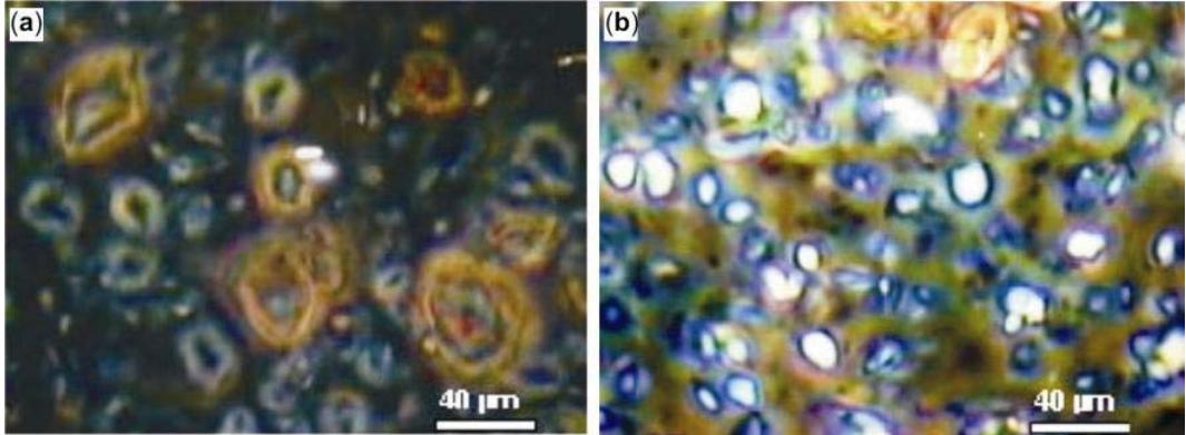
**Figure 3.** Photomicrographs of argillaceous particles (a) before and (b) after compaction (b: particles are carefully taken from the cracking cone surface).
