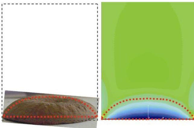
**Figure 5.** Comparison between the cracking cone profile (in red dots) and the stress isovales after compaction.
