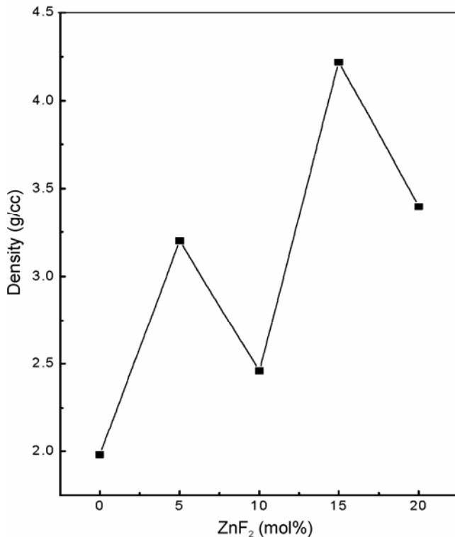
**Figure 1.** Variation of density with ZnF<sub>2</sub> mol%.
