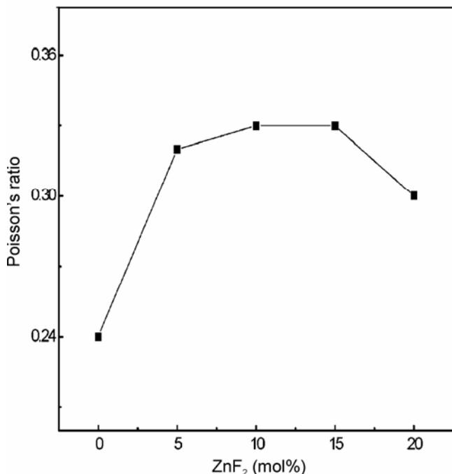
Figure 3. Variation of Poisson's ratio with  $ZnF_2$  mol%.
