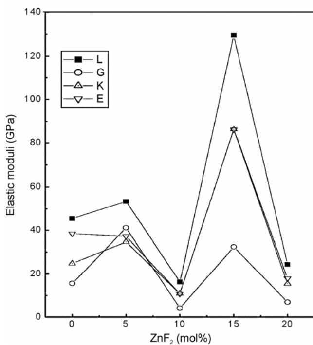
**Figure 2.** Variation of elastic moduli with ZnF<sub>2</sub> mol%.
