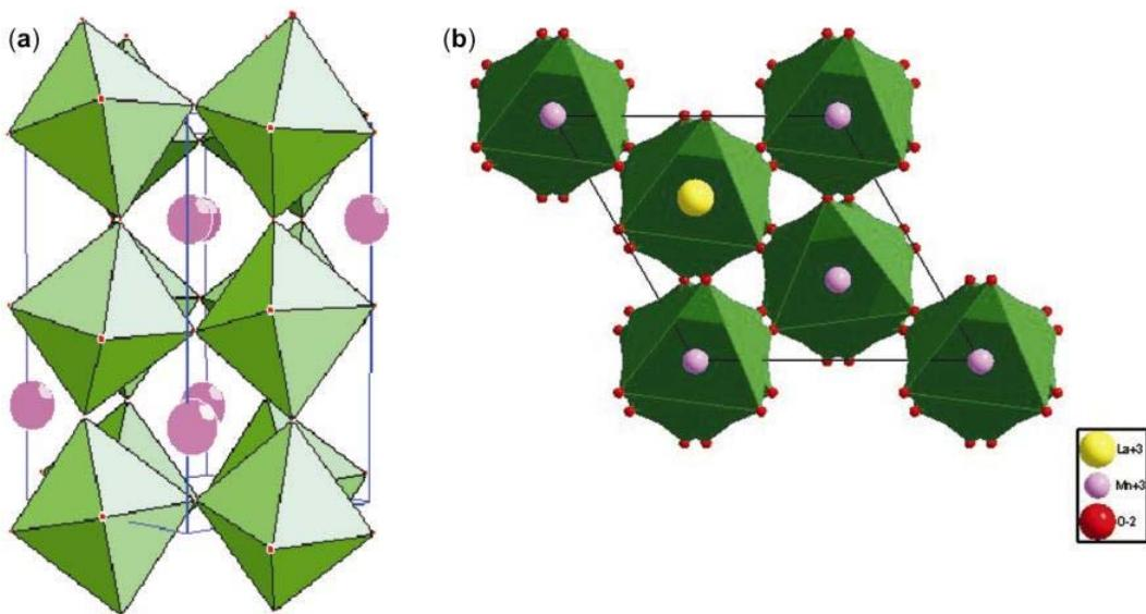
**Figure 4.** Crystal structures of (a) parent  $\text{LaMnO}_3$  in the orthorhombic and (b)  $\text{La}_{0.85}\text{K}_{0.15}\text{MnO}_3$  compound in the rhombohedral structures.
