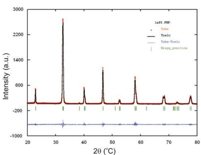
**Figure 3.** Typical observed, calculated and the difference Rietveld refined X-ray diffraction patterns of  $\text{La}_{0.85}\text{K}_{0.15}\text{MnO}_3$  compound.
