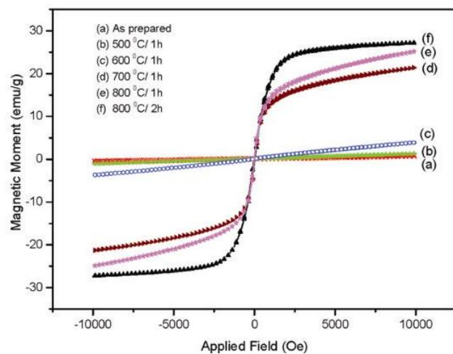
**Figure 8.** Plots of magnetic moment as a function of applied field for  $\text{La}_{0.85}\text{K}_{0.15}\text{MnO}_3$  compounds calcined at different temperatures from  $500$ – $800^\circ\text{C}$  for 1 h.
