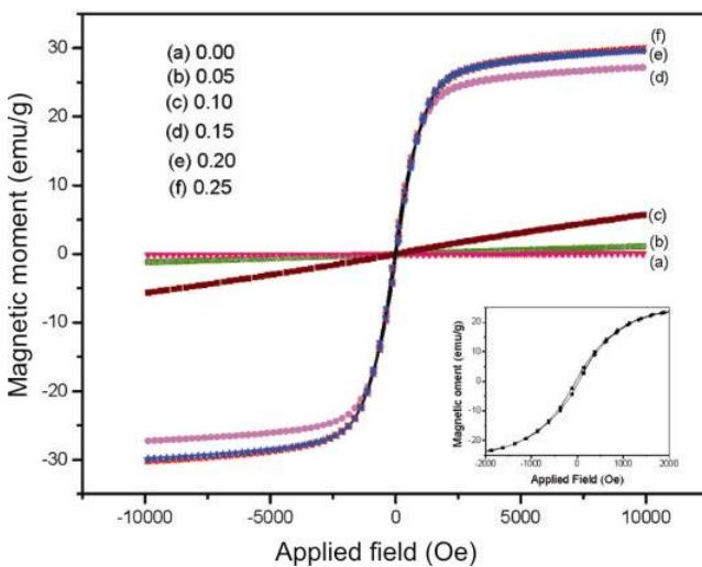
**Figure 9.** Plots of magnetic moment as a function of applied field for  $\text{La}_{1-x}\text{K}_x\text{MnO}_3$  ( $0.00 \leq x \leq 0.25$ ) compounds sintered at  $800^\circ\text{C}$  for 12 h. In the inset, typical hysteresis loop of  $\text{La}_{0.85}\text{K}_{0.15}\text{MnO}_3$  compound is shown.
