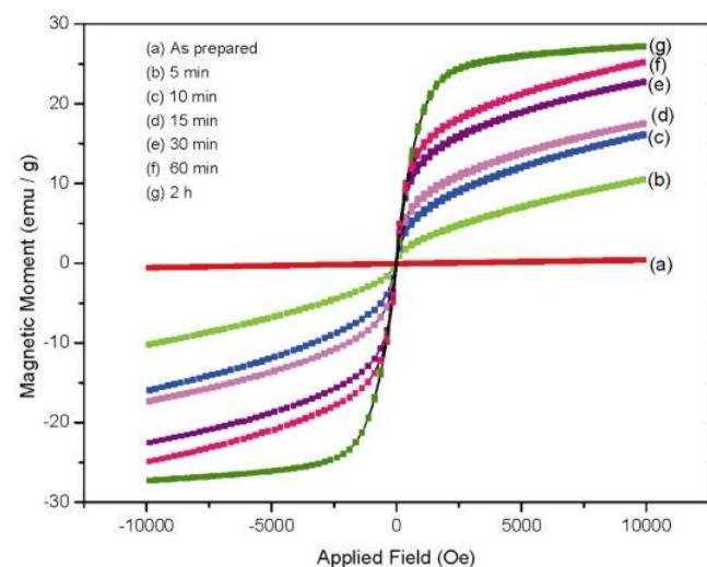
**Figure 7.** Plots of magnetic moment as a function of applied field for  $\text{La}_{0.85}\text{K}_{0.15}\text{MnO}_3$  compounds calcined at  $800^\circ\text{C}$  from 5 min to 2 h.
