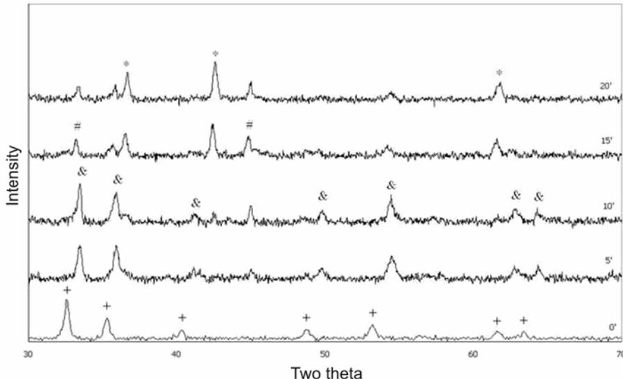
**Figure 1.** The X-ray diffraction patterns of the obtained specimens containing FeTiO<sub>3</sub>-C which was heated in microwave for 5, 10, 15 and 20 min: (TiC (\*), TiO (#), Fe<sub>2</sub>O<sub>3</sub> (&), FeTiO<sub>3</sub> (+)).
