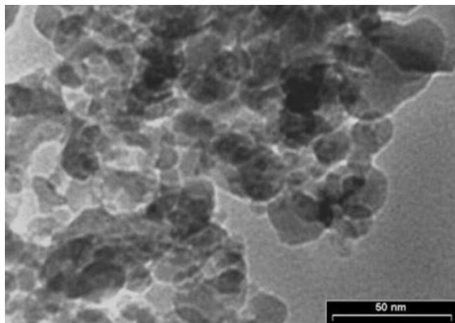
**Figure 7.** The TEM micrograph of sample synthesized with 10%wt Al.
