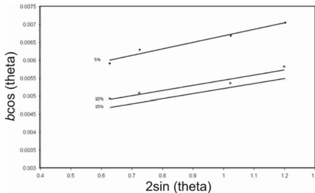
**Figure 6.** Williamson-Hall diagram of the  $\text{FeTiO}_3\text{-C-Al}$  system.
