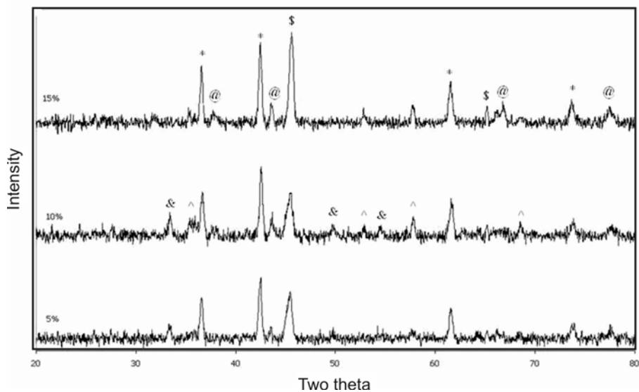
**Figure 5.** X-ray diffraction patterns of the  $\text{FeTiO}_3\text{-C-Al}$  ternary system that was heated in microwave furnace for 20 min with 5, 10 and 15%wt Al (TiC (\*), Fe (\$), SiC (@),  $\text{Al}_2\text{O}_3$  (^),  $\text{Fe}_2\text{O}_3$  (&)).
