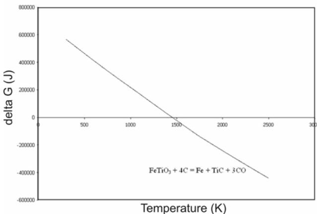
**Figure 2.** The Ellingham–Richardson diagram for the formation reaction of TiC from C and  $\text{FeTiO}_3$ .
