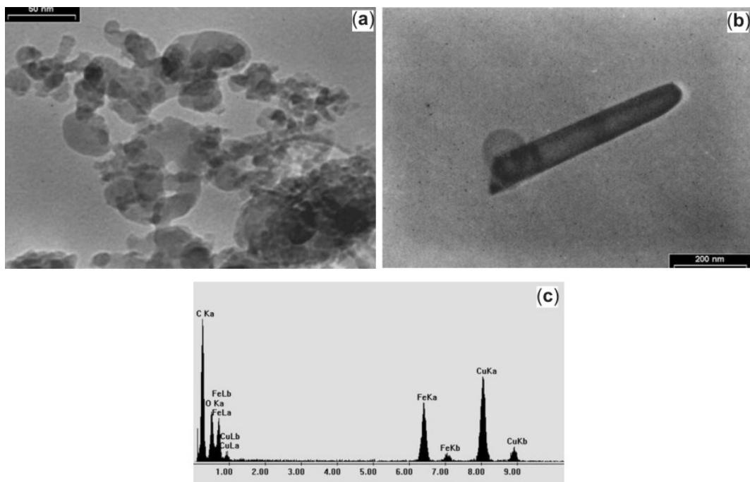
**Figure 4.** (a, b) The TEM microstructures of sample synthesized at 20 min in FeTiO<sub>3</sub>–C and (c) EDS of the marked point in sample b.
