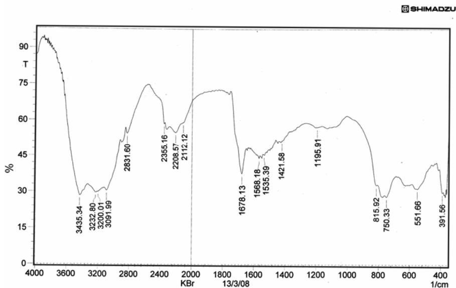
**Figure 4.** FT-IR spectrum of barium calcium iodate.
