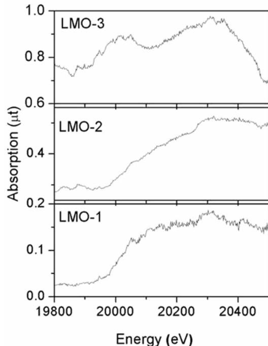
**Figure 4.** X-ray absorption spectra of  $PbMoO_4$  crystals grown under different conditions: (i) stoichiometric grown in air (LMO-1), (ii) stoichiometric grown in argon (LMO-2) and (iii) grown in air from a starting charge containing 1% excess  $PbO$  (LMO-3).
