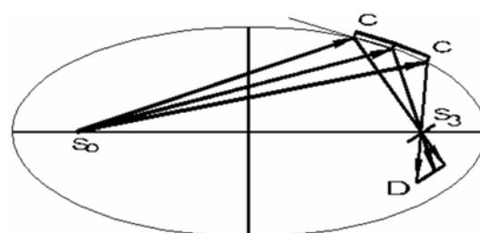
**Figure 1.** Schematic showing the working principle of the dispersive EXAFS beamline (BL-8) at INDUS-2 Synchrotron facility, Indore, India. Where,  $S_0$  is the synchrotron source, CC the crystal,  $S_3$  the sample under investigation and  $D$  the detector.
