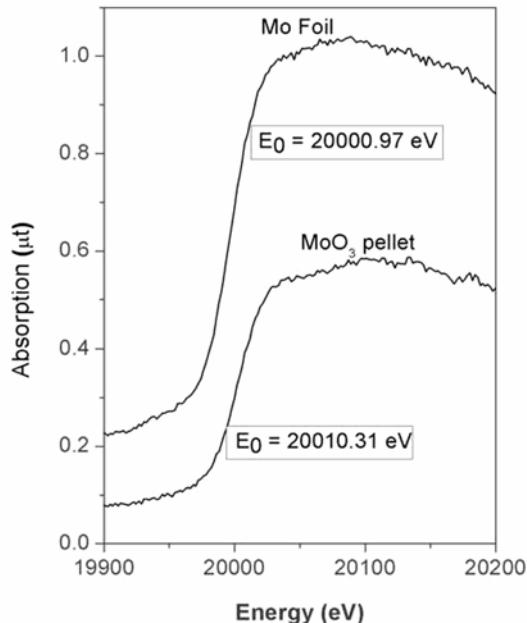
**Figure 3.** X-ray absorption spectra of Mo foil and poly-crystalline  $MoO_3$  around 20,000 eV.
