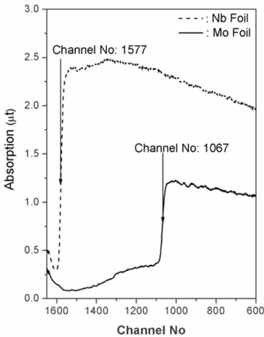
**Figure 2.** X-ray absorption spectra of Nb and Mo foils in the same setting of the crystal bender and detector.
