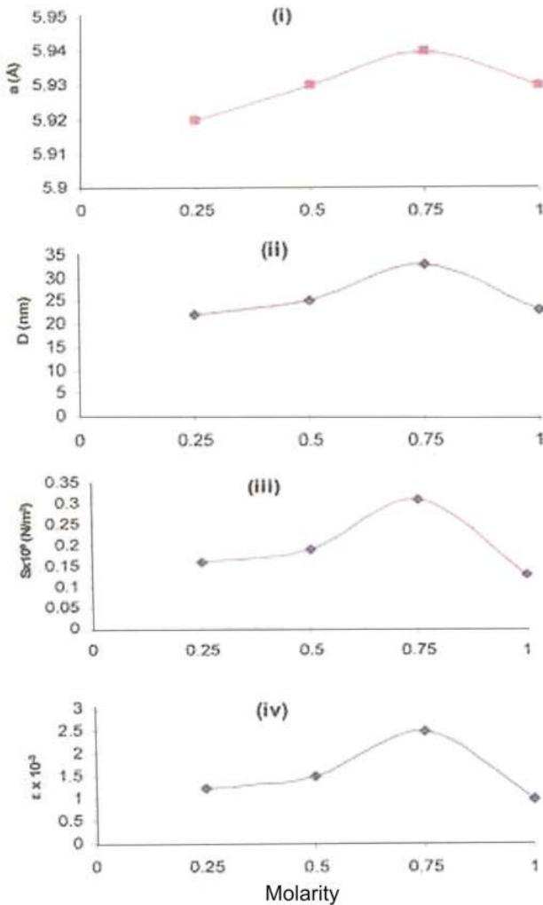
**Figure 3.** Variation of (i) lattice constant, (ii) crystallite size, (iii) average internal stress and (iv) microstrain with molarities in PbS films.
