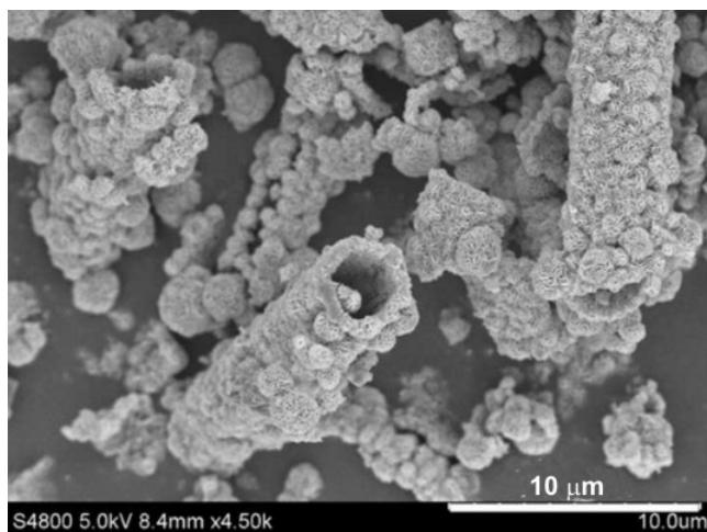
**Figure 5.** SEM image of CuS sample prepared in the absence of ionic liquid.
