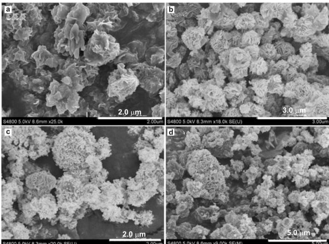
**Figure 4.** SEM images of CuS samples synthesized at different hydrothermal temperatures: **a.** 60, **b.** 70, **c.** 90 and **d.** 100°C.
