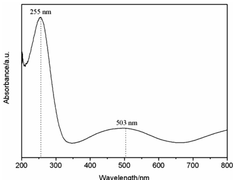
**Figure 3.** UV-Vis absorption spectra of hierarchical CuS flower-like submicrospheres.
