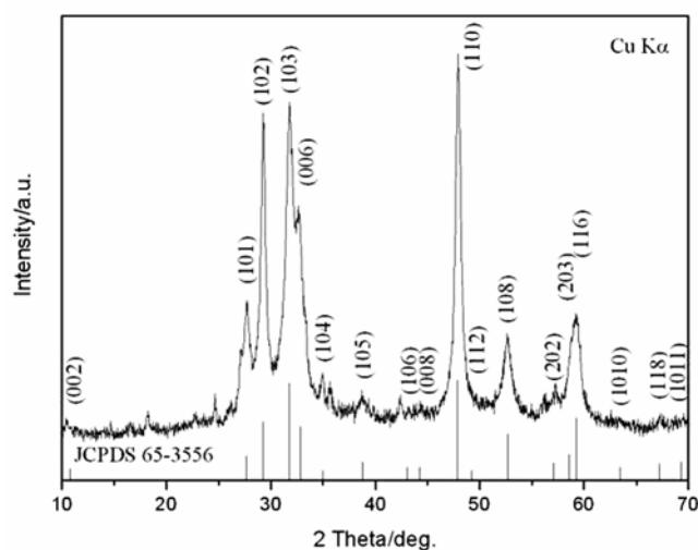
**Figure 1.** Powder X-ray diffraction pattern of hierarchical CuS flower-like submicrospheres.
