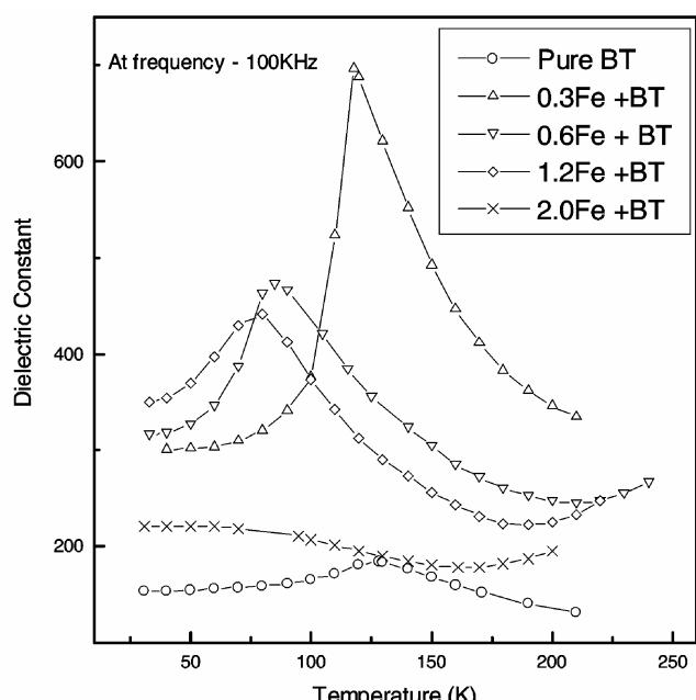
**Figure 3.** Variation of dielectric constant with temperature (at 100 kHz) of undoped and doped (Fe) specimens.
