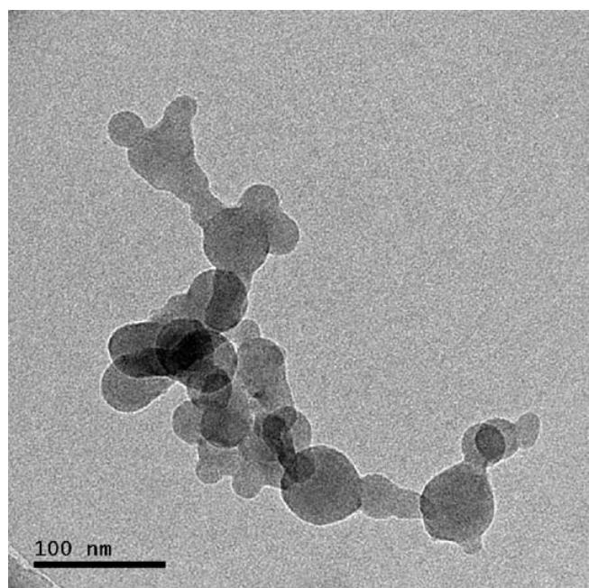
Figure 6. Transmission electron micrograph for 0.6 mole% Ni ion doped BT.
