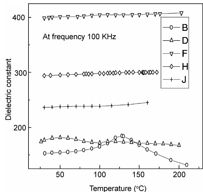
Figure 7. Variation of dielectric constant with temperature (at 100 kHz) of undoped and doped (Ni) specimens.
