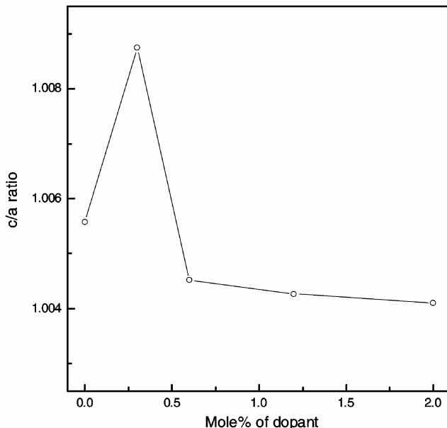
Figure 4. Variation of  $c/a$  ratio with mole% of Fe dopant.
