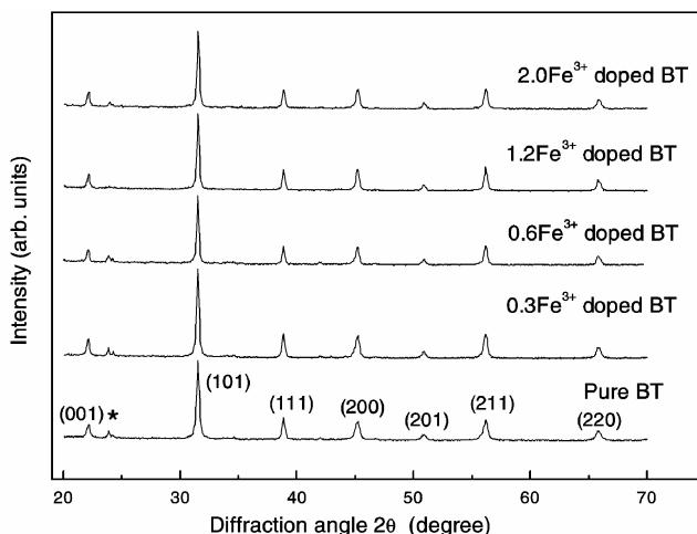
**Figure 1.** XRD pattern of undoped and Fe ion doped BaTiO<sub>3</sub> calcined at 750°C for 2 h.
