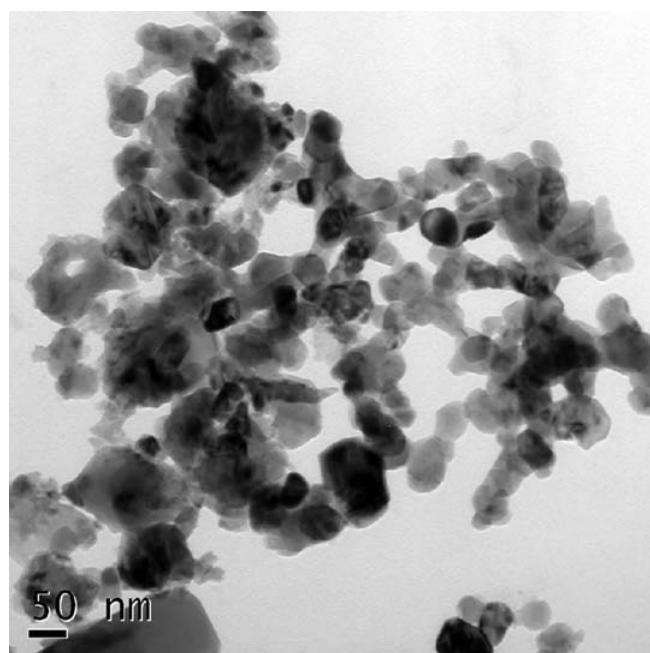
**Figure 2.** Transmission electron micrograph for 0.3 mole% Fe ion doped BaTiO<sub>3</sub>.
