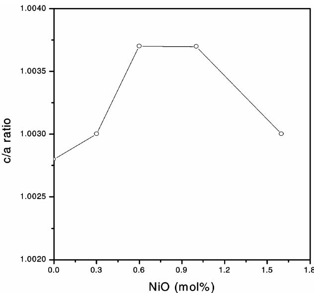
**Figure 8.** Variation of  $c/a$  ratio with the concentration of Ni ions.
