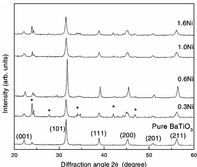
Figure 5. XRD pattern of undoped and Ni ion doped BT.
