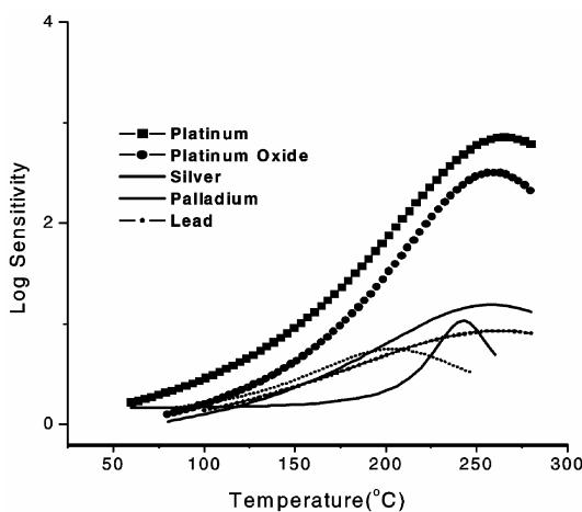
Figure 4. Variation of sensitivity of LPG sensor using various catalysts.
