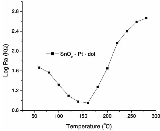
Figure 5. Variation of  $\log R_a$  of LPG sensor with temperature.
