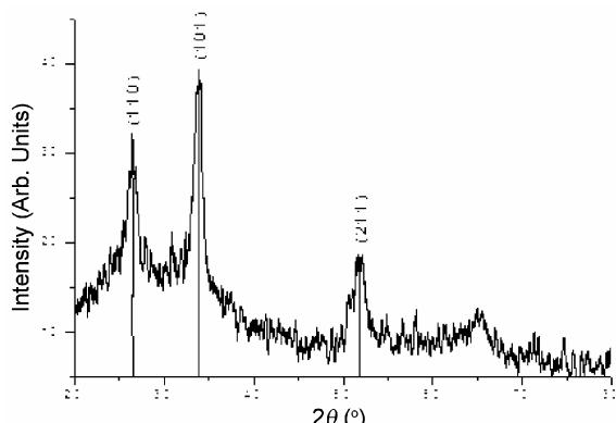
**Figure 2.** XRD pattern of post deposition annealed SnO<sub>2</sub> film (90 nm thick) in air.
