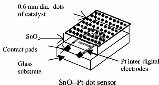
**Figure 1.** Design of dotted metal/SnO<sub>2</sub> LPG sensor.
