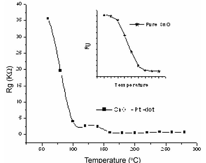
Figure 6. Variation of  $\log R_g$  of LPG sensor with temperature.
