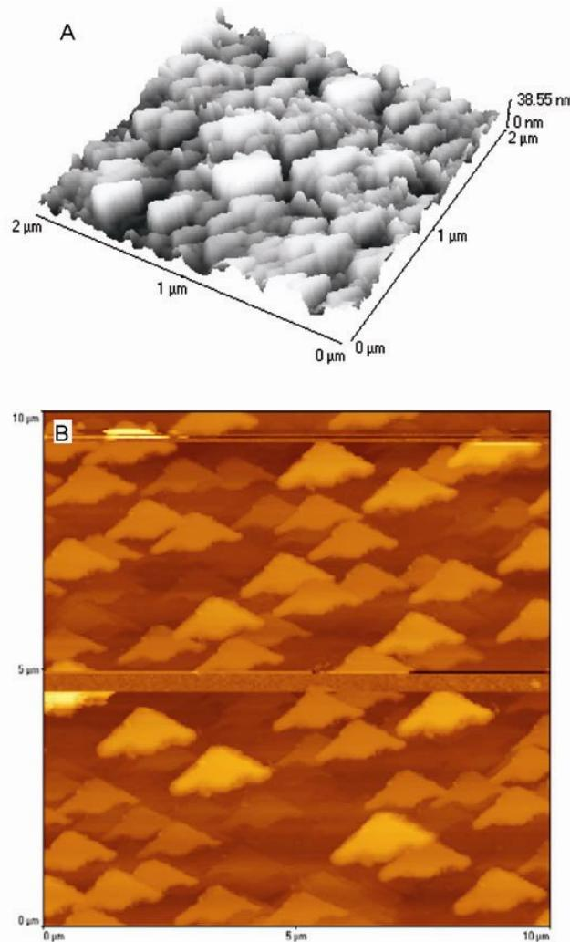
**Figure 3.** **A.** AFM image of post deposition annealed SnO<sub>2</sub> film and **B.** AFM image of SnO<sub>2</sub>-Pt dotted sensor structures.
