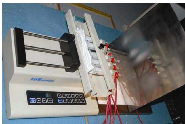
Figure 1. Multi syringe setup for electrospinning with a stationary collecting electrode.
