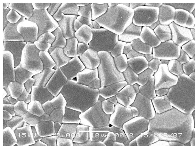
**Figure 3.** SEM micrograph of NBT–NBZN0.015 ceramic sintered at 1190°C for 2 h.
