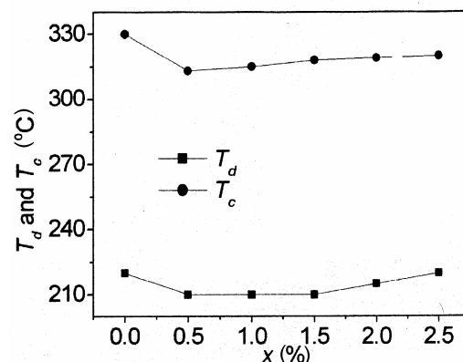
Figure 6. Depolarization temperature,  $T_d$ , and Curie temperature,  $T_c$ , of NBT–NBZN<sub>x</sub> ceramics as a function of  $x$ .
