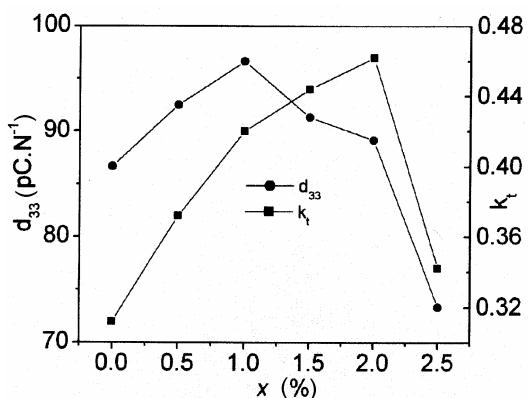
Figure 4. Piezoelectric constant,  $d_{33}$  and thickness electromechanical coupling factor,  $k_t$ , of NBT–NBZN<sub>x</sub> ceramics as a function of  $x$ .
