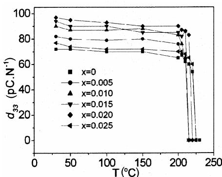
Figure 5. Temperature dependence of piezoelectric constant,  $d_{33}$ , of NBT–NBZN<sub>x</sub> ceramics.
