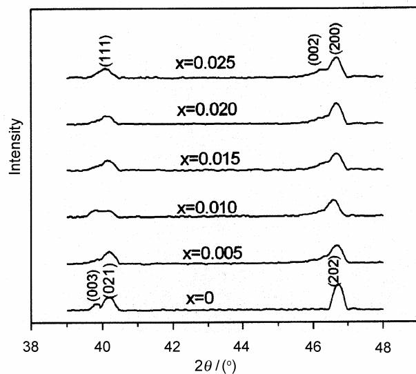
**Figure 2.** XRD patterns of NBT–NBZN<sub>x</sub> ceramics in  $2\theta$  range of 39–48°.
