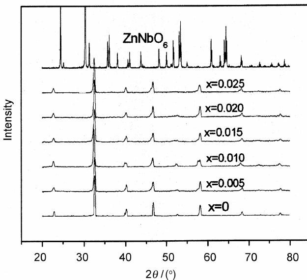
**Figure 1.** The XRD patterns of  $\text{ZnNb}_2\text{O}_6$  powder and NBT–NBZN<sub>x</sub> ceramics.
